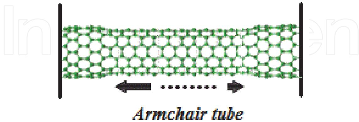
Fig. 13. Schematic view of a carbon nanotube quantum dot.
