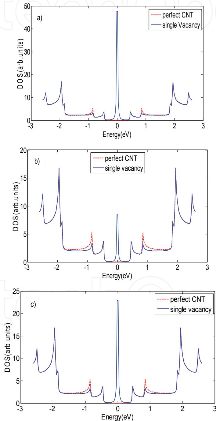
Fig. 7. The density of states of finite zigzag carbon nanotubes (11,0) in presence of the single vacancy in a: 2<sup>th</sup> ring b: 3<sup>th</sup> ring c: 4<sup>th</sup> ring of 4<sup>th</sup> mode
