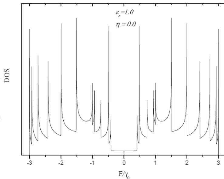
Fig. 2. Density of states for a pure (12, 0) SWCNT
