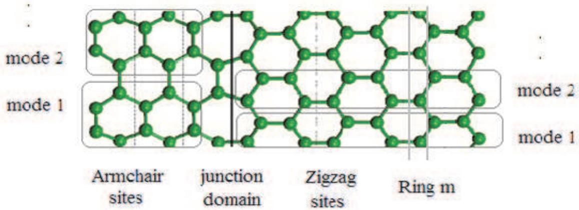
Fig. 14. Schematic representation of Armchair and zigzag modes and rings in real space, a pentagon-heptagon ring as a junction between zigzag and armchair carbon nanotubes quantum dots are shown.
