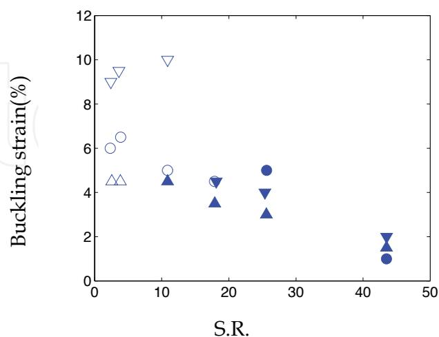
Fig. 6. The relationship between the buckling strain and slenderness ratio for zigzag CNTs.  $\nabla\nabla$ : (9,0),  $\circ\bullet$ : (14,0),  $\triangle\blacktriangle$ : (17,0) CNT.
