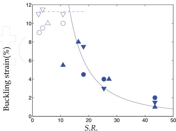
Fig. 8. The comparisons between the continuum predictions and molecular simulation results for CNTs. ▽▼:(5,5), ○●:(9,0) and △▲:(6,4)
