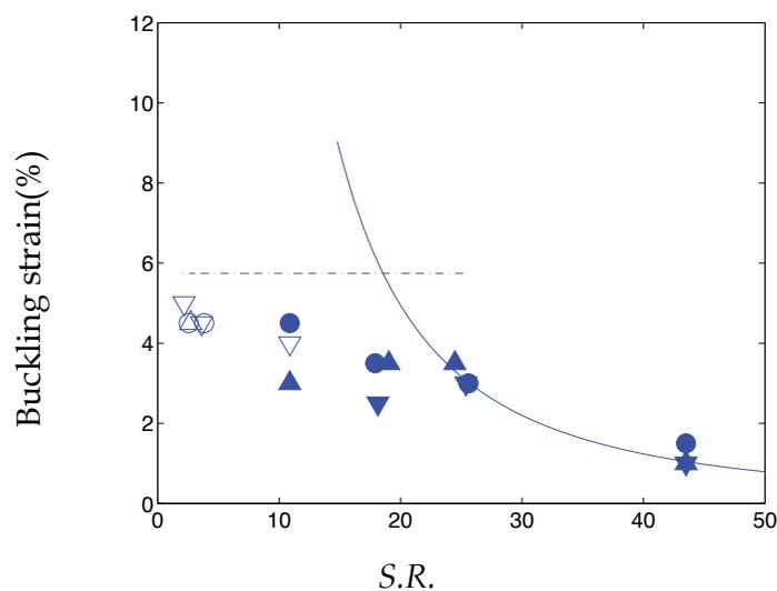
Fig. 10. The comparisons between the continuum predictions and molecular simulation results for CNTs.  $\nabla$  $\blacktriangledown$ : (10,10),  $\circ$  $\bullet$ : (17,0) and  $\triangle$  $\blacktriangle$ : (12,8)
