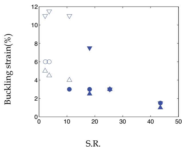
Fig. 5. The relationship between the buckling strain and slenderness ratio for armchair CNTs.  $\nabla\nabla$ : (5,5),  $\circ\bullet$ : (8,8),  $\triangle\blacktriangle$ : (10,10) CNT.
