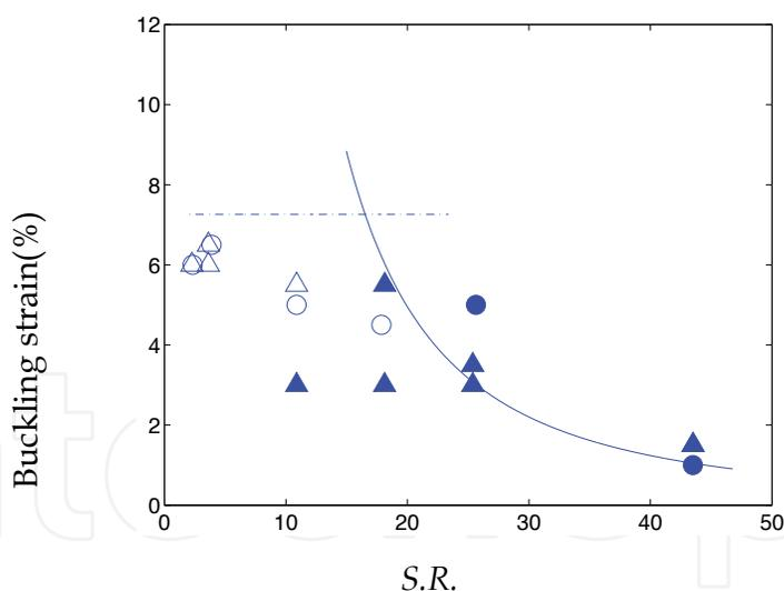
Fig. 9. The comparisons between the continuum predictions and molecular simulation results for CNTs. ▽▼:(8,8), ○●:(14,0) and △▲:(9,6)
