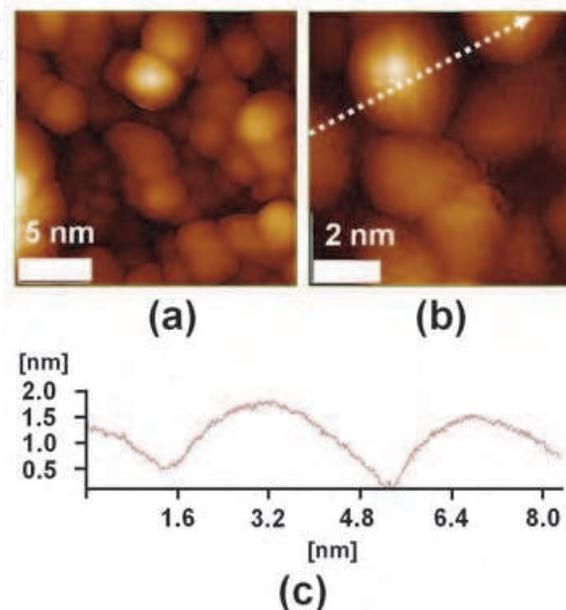
Fig. 7. (a) and (b) STM image of the cap structures produced on 6H-SiC(000-1) substrates after heating at 1250°C in a vacuum electric furnace. (c) Height profile of cap structures in the direction marked by an arrow in (b).
