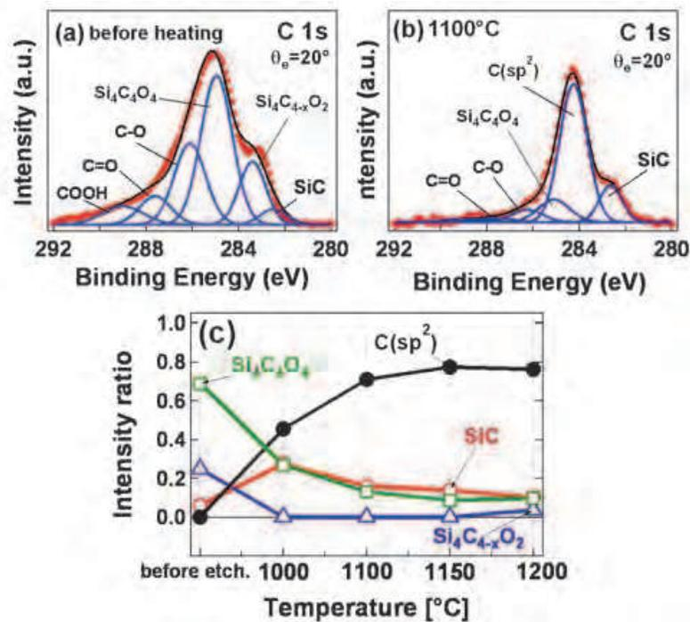
Fig. 5. XPS spectra of SiC(000-1) surface of (a) before heating (after HF etching), and (b) after heating at 1100°C in UHV. Both spectra were measured at the take-off angle of  $20^\circ$  from the surface plane. (c) Temperature dependence of relative intensities of each component in XPS spectra.
