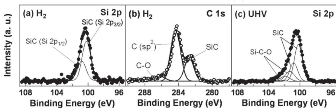
Fig. 14. (a) Si 2p and (b) C 1s XPS spectra for 6H-SiC(000-1) substrates after annealing at 1250°C in a hydrogen atmosphere of  $10^{-2}$  Pa. (c) Si 2p XPS spectrum for 6H-SiC(000-1) substrates after annealing in a UHV. All spectra were deconvoluted into a set of Gaussian peaks after implementing background subtraction that accounted for previous XPS spectra of SiC (Hornetz et al., 1995).
