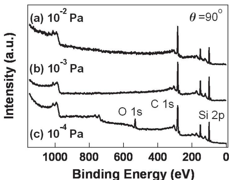
Fig. 13. XPS survey spectra for 6H-SiC(000-1) substrates after annealing at  $1250^\circ\text{C}$  in a hydrogen atmosphere of: (a)  $10^{-2}$ , (b)  $10^{-3}$  and (c)  $10^{-4}$  Pa.
