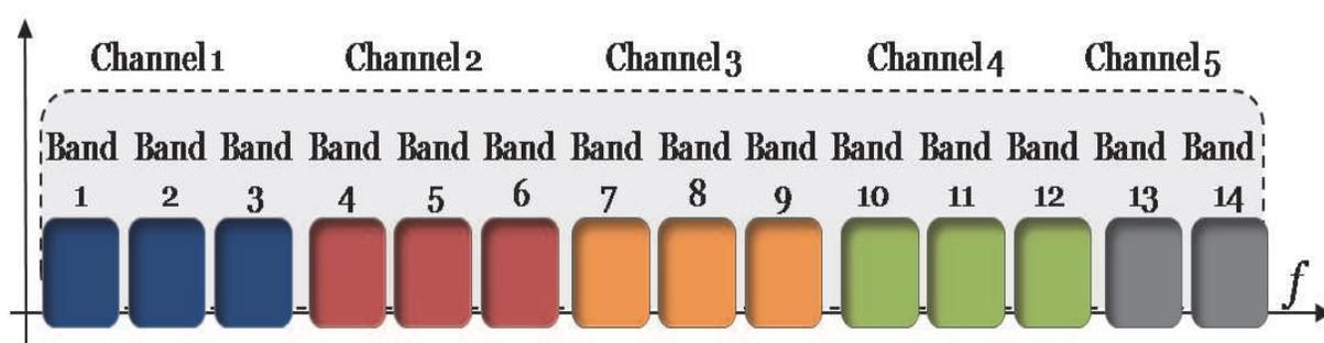
Fig. 1. UWB spectrum bands in the MB-OFDM system.
