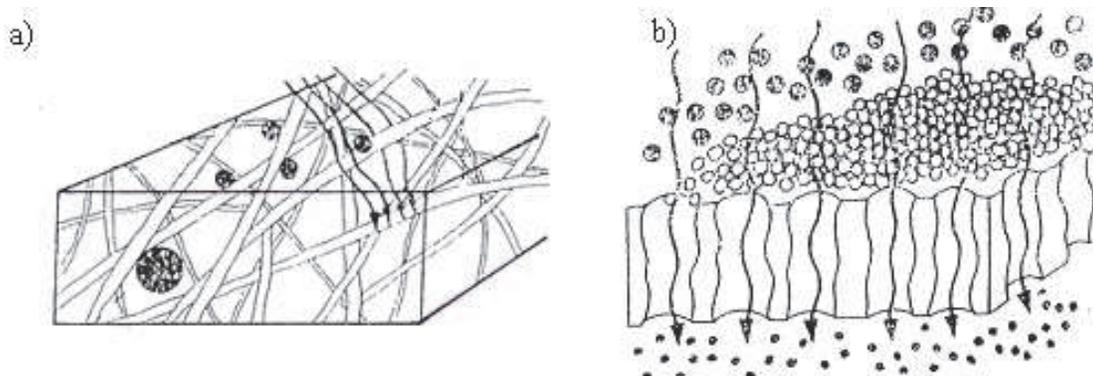
Fig. 1. Filtrations mechanisms
