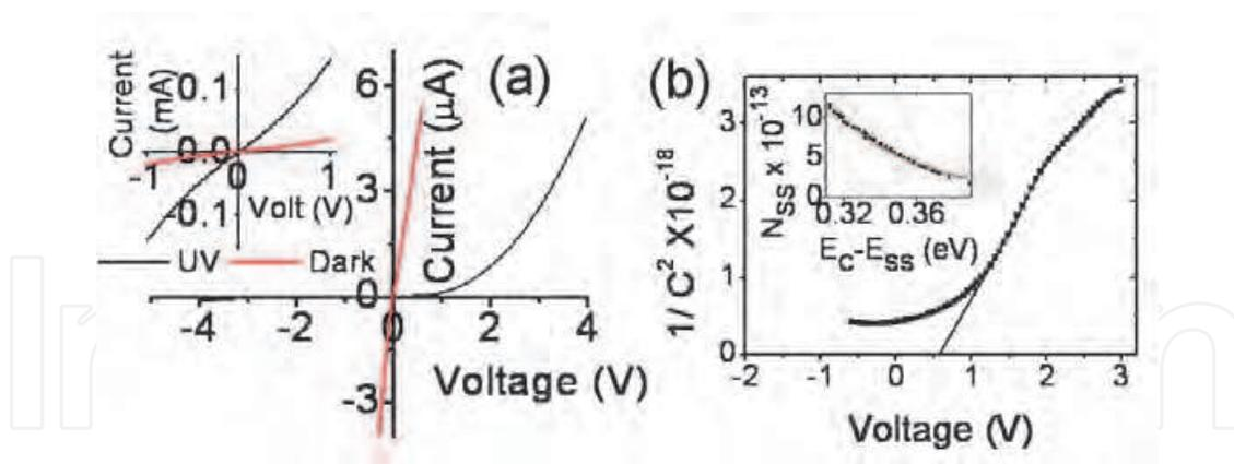
Fig. 9. (a)  $I$ - $V$  characteristics for a representative Au/ZnO nanowire Schottky diode before and after UV illumination. The inset shows the  $I$ - $V$  characteristics of a device with both side ohmic contacts. (b) Plot of  $(1/C^2)$  with  $V$  for Au/ZnO nanowires Schottky diode. The inset shows the density of interface states as a function of interface state energy ( $E_C - E_{SS}$ ).
