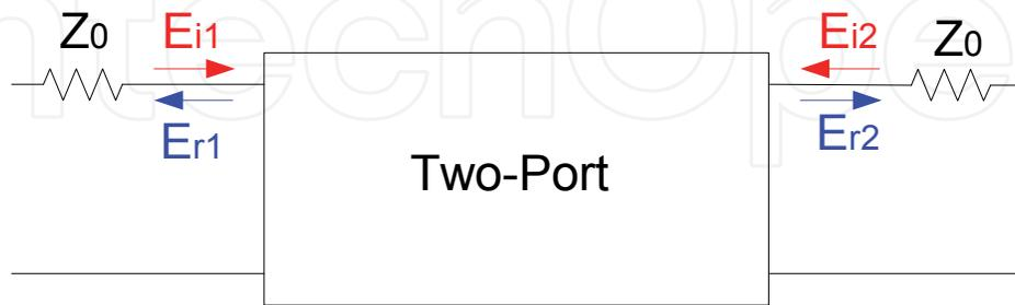
Fig. 7. Two port circuit representation for S-parameters.
