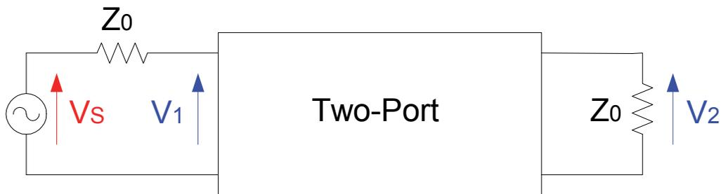
Fig. 8. Circuit topology used to measure S-Parameters.
