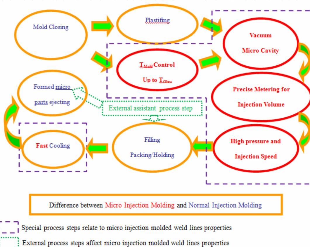
Fig. 1-2. Micro injection molding processing steps
