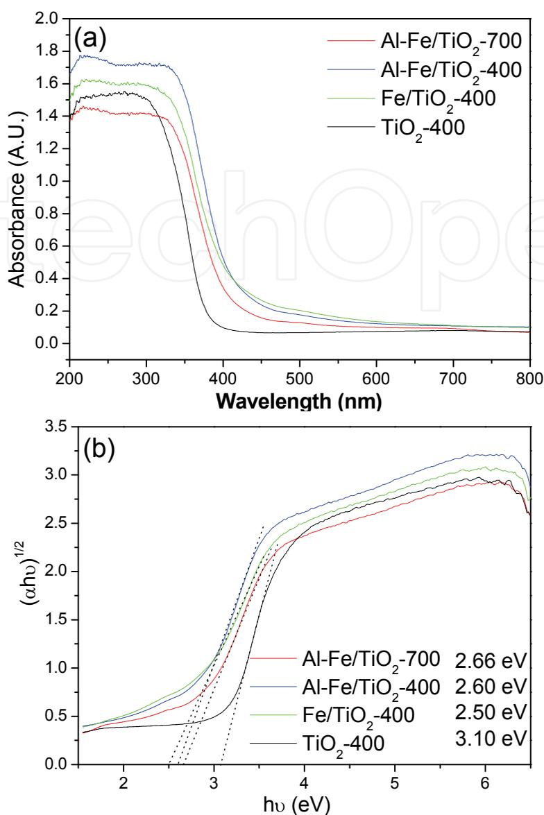
Fig. 4. UV-visible absorption spectra of (a) and determination of indirect interband transition energies (b) for pure TiO<sub>2</sub>, Fe/TiO<sub>2</sub>-400, Al-Fe/TiO<sub>2</sub>-400, and Al-Fe/TiO<sub>2</sub>-700 samples.
