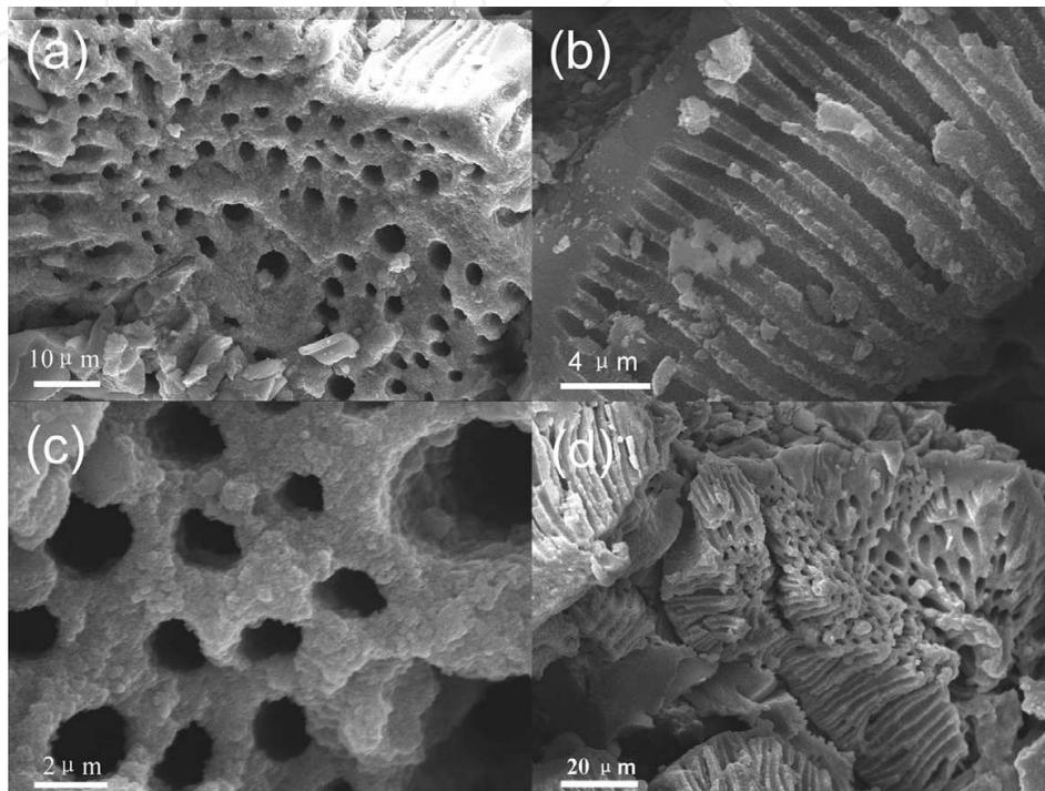
Fig. 3. SEM images of the Al-Fe/TiO<sub>2</sub> samples calcined at 400 °C (a, b, c), and 600 °C (d).
