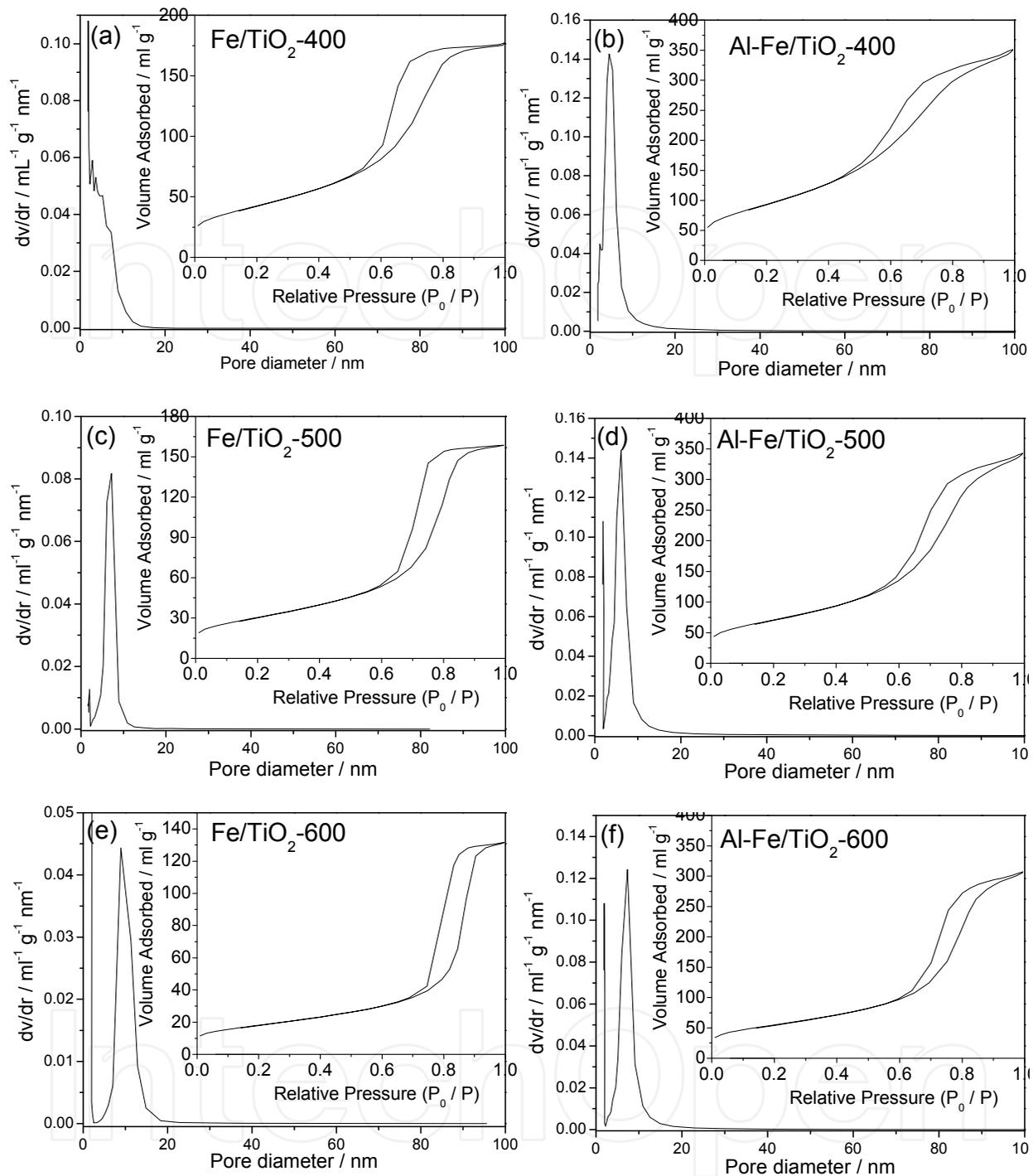
Fig. 2. N<sub>2</sub> adsorption-desorption isotherms (a, c, and e) and pore size distributions (b, d, and f) of the as-prepared Fe/TiO<sub>2</sub> and Al-Fe-TiO<sub>2</sub> samples calcined at different temperatures.
