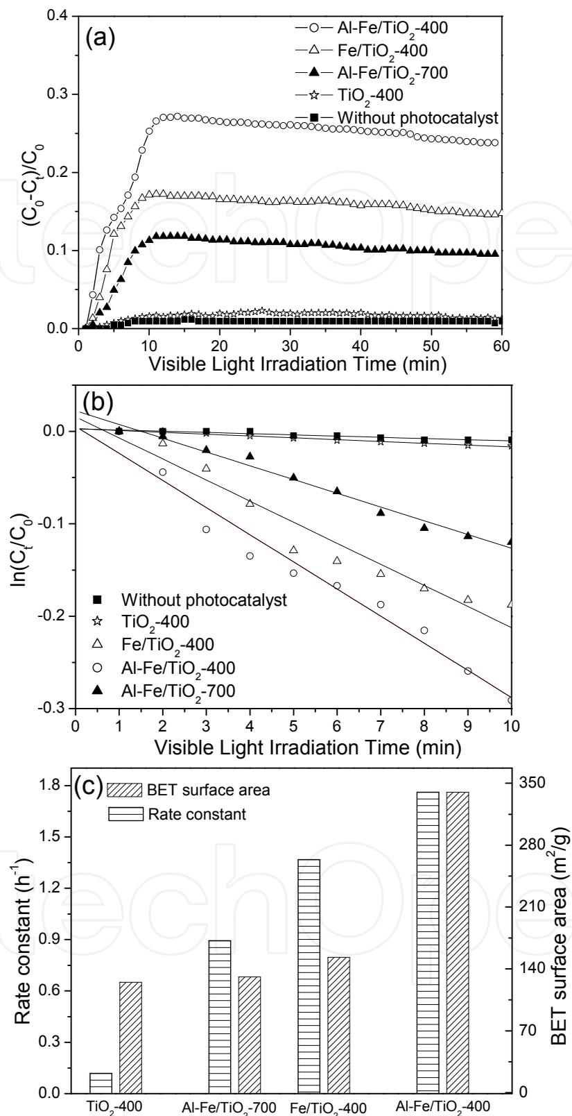
Fig. 5. (a) Plots of the removal of NO concentration vs irradiation time in the presence of the as-prepared products with visible-light irradiation ( $\lambda > 400$  nm). (b) Dependence of  $\ln(C_t/C_0)$  on irradiation time. (c) Relationship between rate constant and BET surface area over the as-prepared products.
