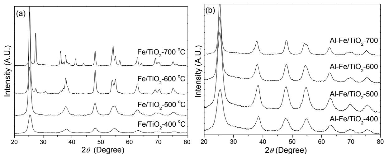
Fig. 1. XRD patterns of the as-prepared Fe/TiO<sub>2</sub> and Al-Fe/TiO<sub>2</sub> samples calcined at different temperatures.
