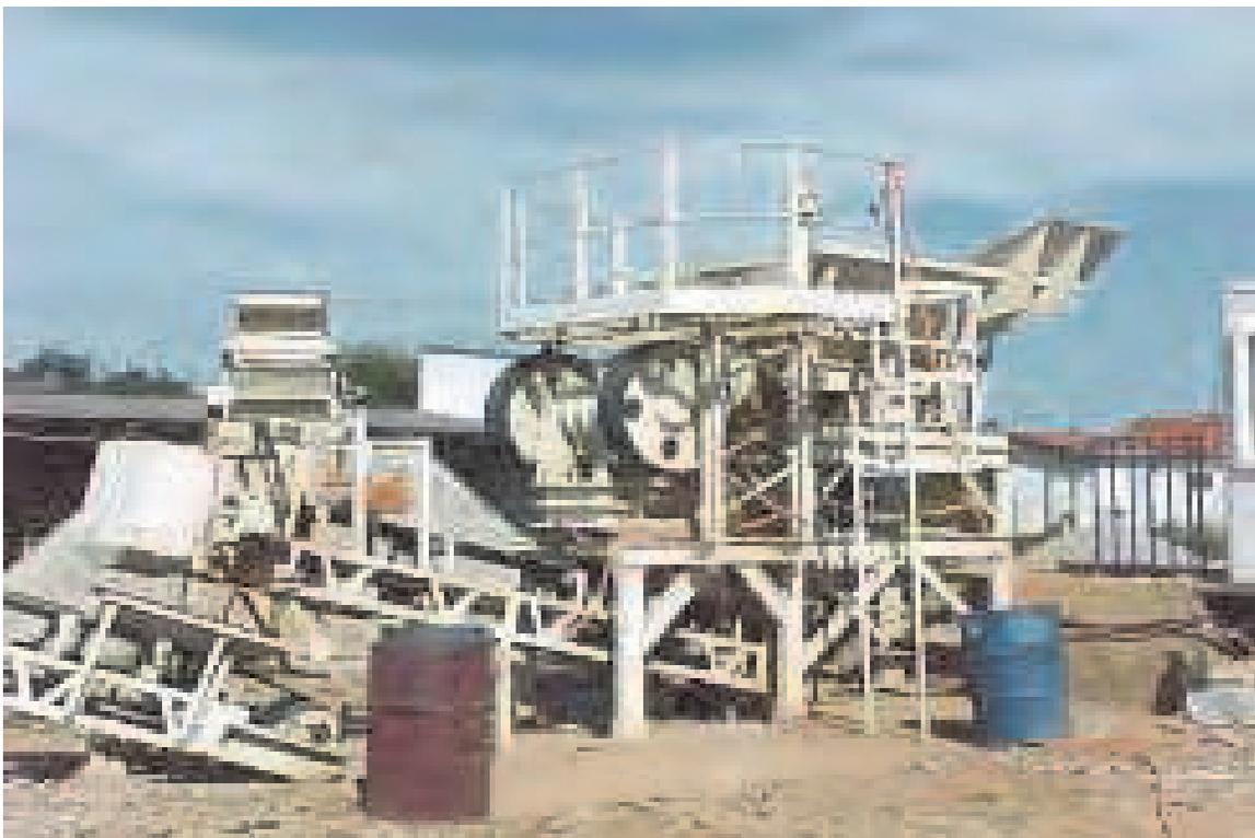
Fig. 7. Plant equipment: a set vibrating feeder jaw crusher + + belt
