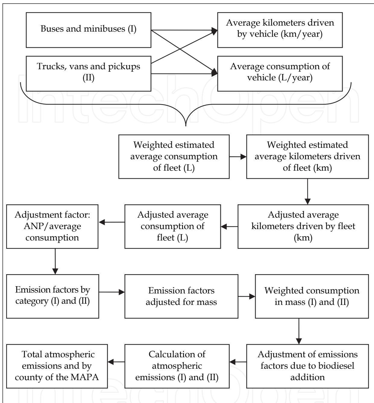
Fig. 3. Block chart of the calculation system
