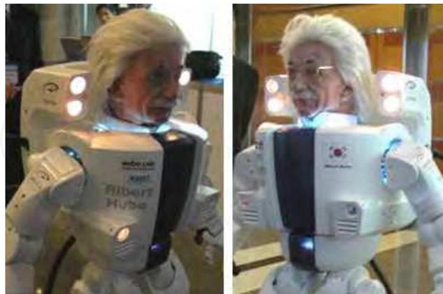
Figure 20. The lights around the head and those of the shoulder connection, and the front of the waist
