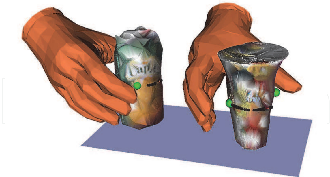
Fig. 9. The rotation axis of the hand is defined by the fingertip of the thumb and the index finger of the gripper. This rotation axis must be aligned with the axis defined by the grasping points. The calculated grasping pose of the gripper is by object no. 8 (Cappy) -32.5^\circ and object no. 9 (Smoothie) -55^\circ .
