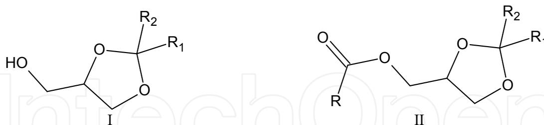
Fig. 2.2. Structure of intermediate I and product II (R =15-17 carbons; R<sub>1</sub>, R<sub>2</sub> = CH<sub>3</sub>)
