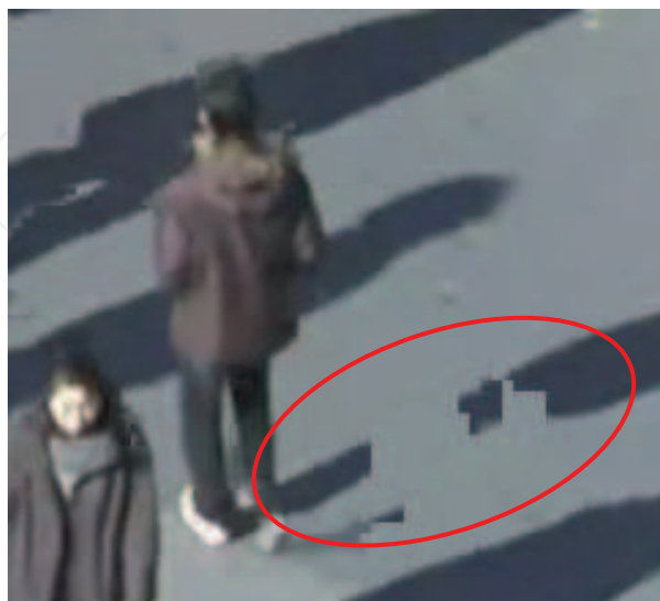
Fig. 9. Detail of the interpolated frame \hat{F}_0 of the PeopleOnStreet sequence. Failed motion compensation is highlighted in red.
