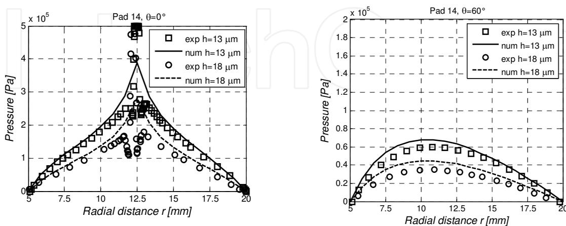
Fig. 30. Comparison of experimental and numerical radial pressure distributions, pad "14",  $p_s = 0.5$  MPa, orifice diameter  $d = 0.2$  mm, pocket diameter  $d_0 = 4$  mm, pocket depth  $\delta = 0$   $\mu$ m, air gap height  $h = 13$  and  $18$   $\mu$ m,  $\theta = 0^\circ$  and  $60^\circ$ ,  $n \times m = 21 \times 72$ .
