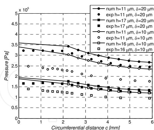
Fig. 27. Numerical and experimental circumferential pressure distribution across pad number "11", type "c", supply pressure  $p_s = 0.5$  MPa, orifice diameter  $d = 0.2$  mm, pocket diameter  $d_0 = 4$  mm, pocket depth  $\delta = 10$  and  $20 \mu\text{m}$ ,  $n \times m = 20 \times 20$ .
