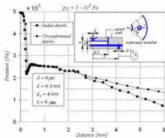
Fig. 13. Radial and circumferential pressure distribution across pad number "12", type "c", supply pressure  $p_S = 0.5$  MPa, orifice diameter  $d = 0.3$  mm, pocket diameter  $d_0 = 4$  mm, pocket depth  $\delta = 0$   $\mu\text{m}$ .
