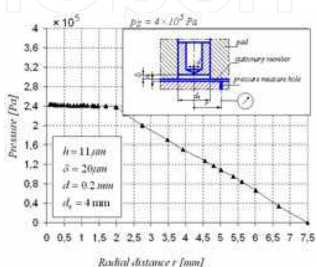
Fig. 11. Radial pressure distribution across pad number "11", type "c", supply pressure  $p_s = 0.4$  MPa.
