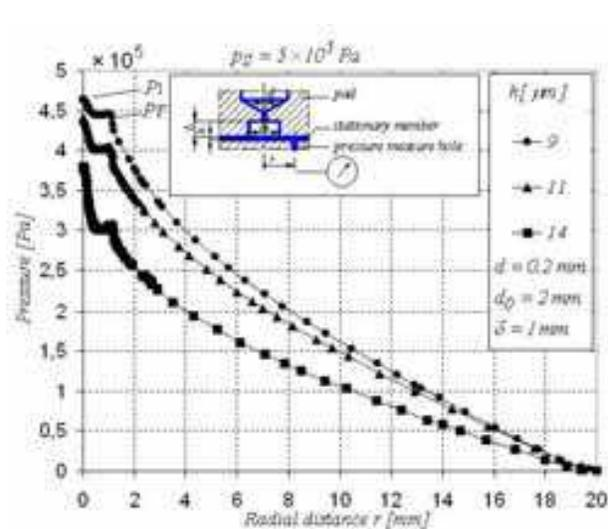
Fig. 9. Radial pressure distribution across the entire pad number "8", type "b", supply pressure  $p_s = 0.5$  MPa.
