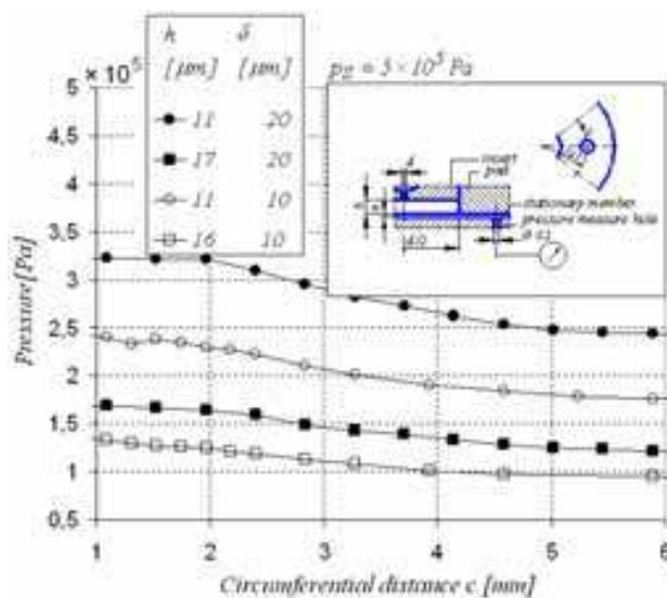
Fig. 12. Circumferential pressure distribution across pad number "11", type "c", supply pressure  $p_S = 0.5$  MPa, orifice diameter  $d = 0.2$  mm, pocket diameter  $d_0 = 4$  mm, pocket depth  $\delta = 10$  and  $20$   $\mu\text{m}$ .
