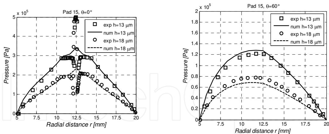
Fig. 31. Comparison of experimental and numerical radial pressure distributions, pad "15",  $p_s = 0.5$  MPa, orifice diameter  $d = 0.3$  mm, pocket diameter  $d_0 = 4$  mm, pocket depth  $\delta = 10\mu\text{m}$ , air gap height  $h = 13$  and  $18\mu\text{m}$ ,  $\theta = 0^\circ$  and  $60^\circ$ ,  $n \times m = 21 \times 72$ .
