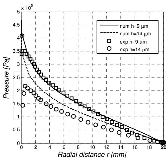
Fig. 24. Numerical and experimental radial pressure distribution across number "1" pad, type "a", supply pressure  $p_s = 0.5 \text{ MPa}$ , orifice diameter  $d = 0.2 \text{ mm}$ , air gap height  $h = 9$  and  $14 \mu\text{m}$ ,  $n \times m = 20 \times 20$ .
