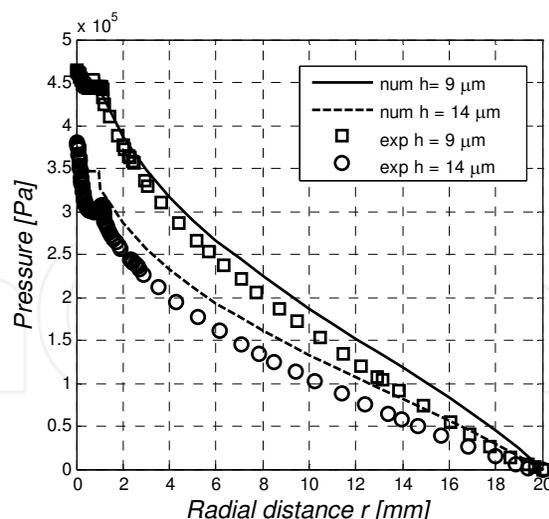
Fig. 25. Numerical and experimental radial pressure distribution across entire pad number "8", type "b", supply pressure  $p_s = 0.5 \text{ MPa}$ , orifice diameter  $d = 0.2 \text{ mm}$ , pocket diameter  $d_0 = 2 \text{ mm}$ , pocket depth  $\delta = 1 \text{ mm}$ , air gap height  $h = 9$  and  $14 \mu\text{m}$ ,  $n \times m = 20 \times 20$ .
