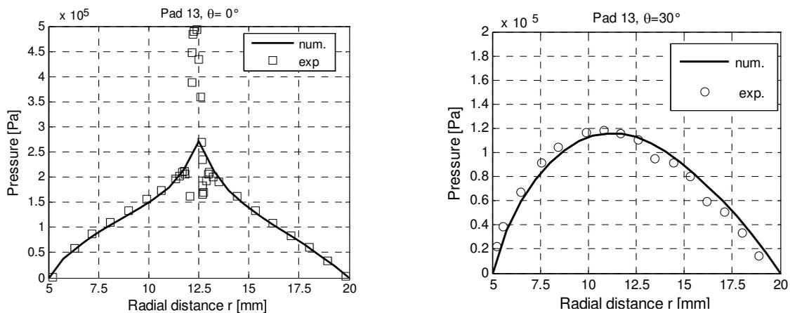
Fig. 29. Numerical and experimental circumferential pressure distribution across pad "13", supply pressure  $p_s = 0.5$  MPa, orifice diameter  $d = 0.2$  mm, pocket diameter  $d_0 = 4$  mm, pocket depth  $\delta = 0$   $\mu$ m, air gap height  $h = 15$   $\mu$ m,  $\theta = 0^\circ$  and  $30^\circ$ ,  $n \times m = 21 \times 72$ .
