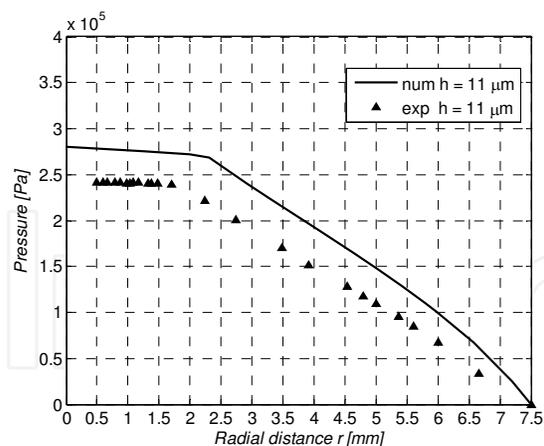
Fig. 26. Radial pressure distribution across pad number "11", type "c", supply pressure  $p_s = 0.4$  MPa, orifice diameter  $d = 0.2$  mm, pocket diameter  $d_0 = 4$  mm, pocket depth  $\delta = 20 \mu\text{m}$ , air gap height  $h = 11 \mu\text{m}$ ,  $n \times m = 20 \times 20$ .
