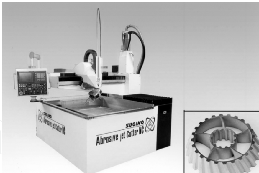
Fig. 2. Modern five-axis water jet machining system and sample part manufactured by the system (Sugino Machine Ltd., 2007)
