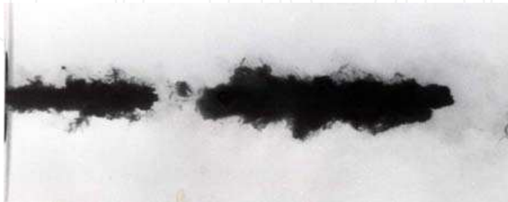
Fig. 6. Cavitating jet at p_i = 69 MPa and \sigma = 0.006 (flow direction is from left to right)
