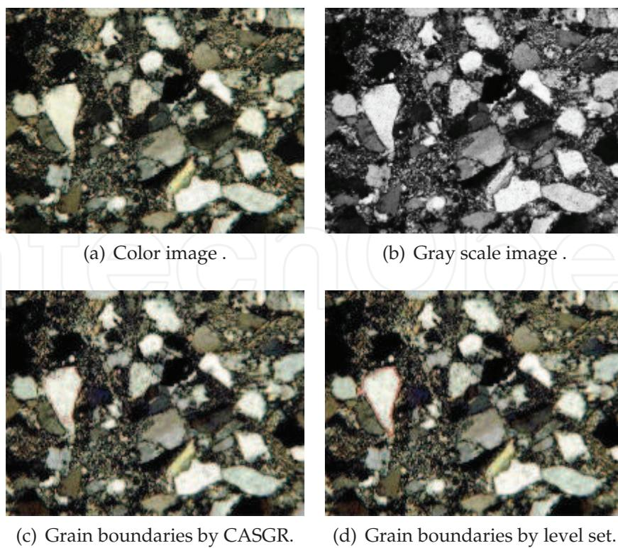
Fig. 5. Grain boundaries detection of low strain sample.
