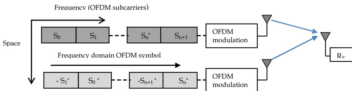
Fig. 4. Space-Frequency Block Coding SFBC assuming two antennas
