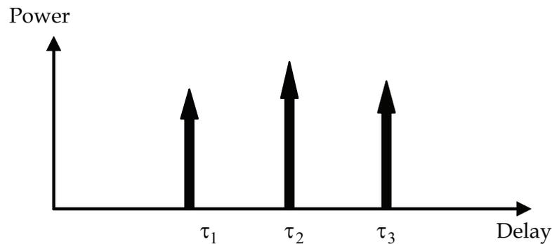
Fig. 2. Power delay profile of a multipath channel
