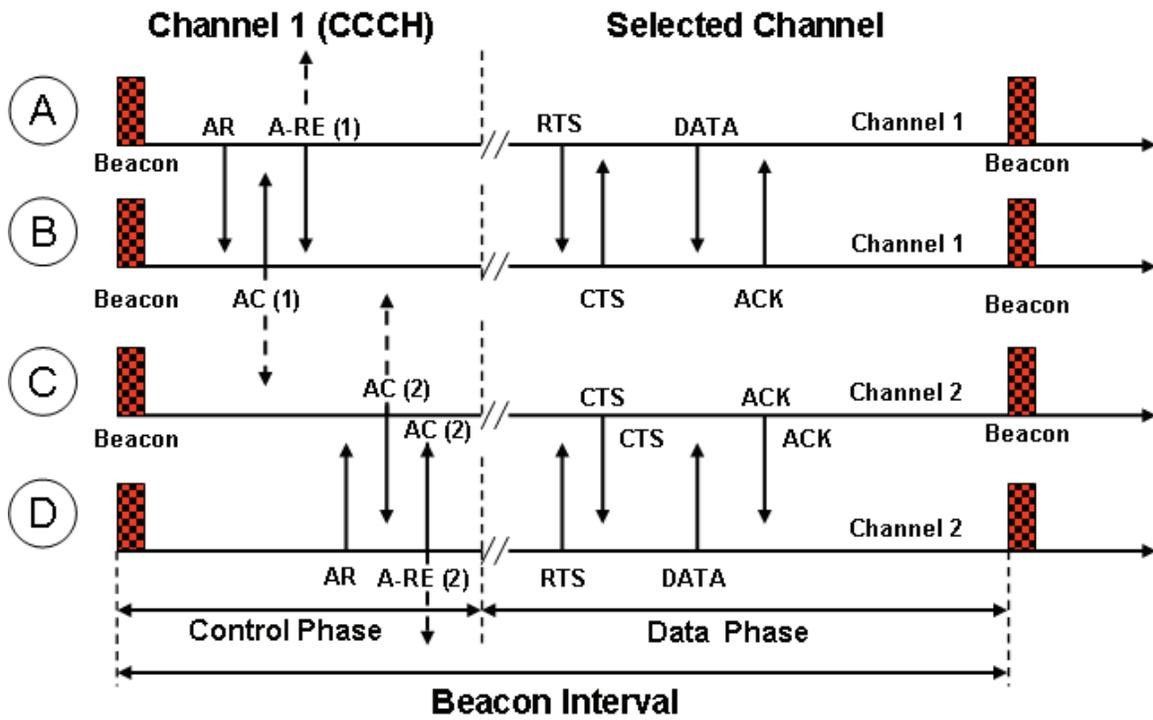
Fig. 8. MMAC protocol (figure inspired from [so04])
