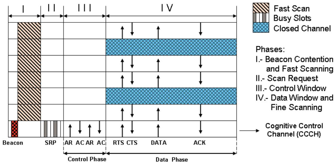
Fig. 9. MMAC-CR protocol (figure inspired from [timms07])
