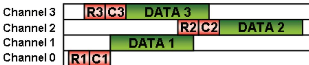
Fig. 5. Common Hopping Approach (figure inspired from [mo07])
