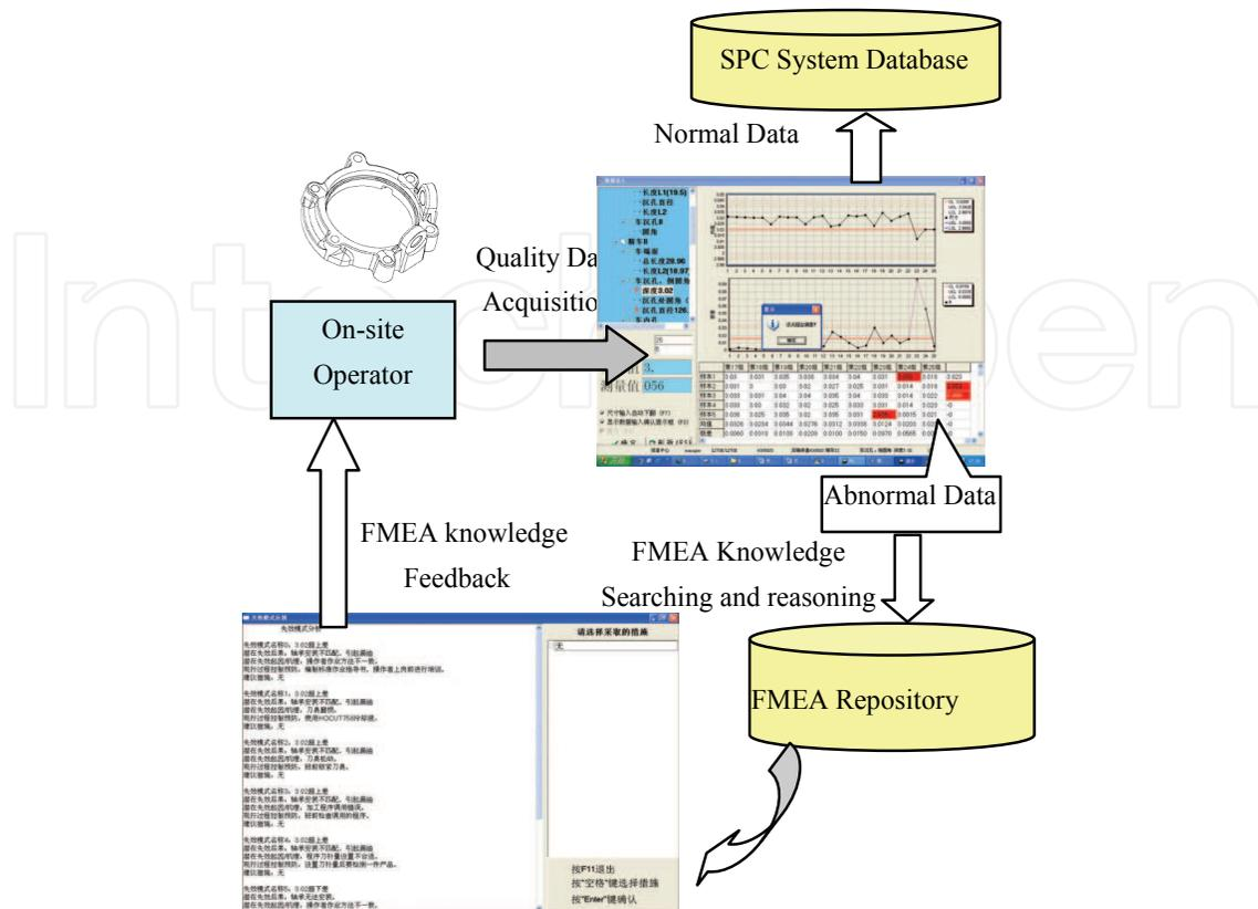
Fig. 2. A specific quality control process based on FMEA repository and SPC system
