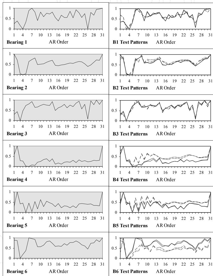
Fig. 8. AR parameters patterns of defective bearings
