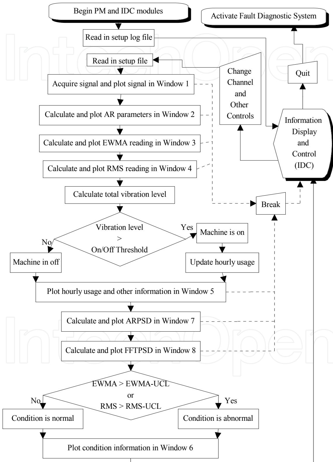
Fig. 3. Flowchart of PM and IDC modules
