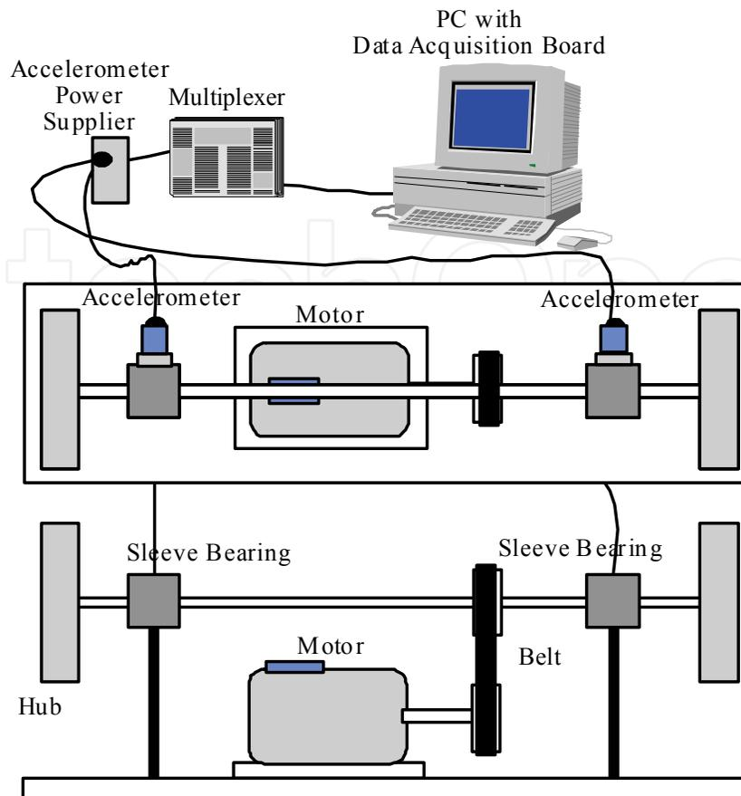
Fig. 5. The test rig for ISDS experiment
