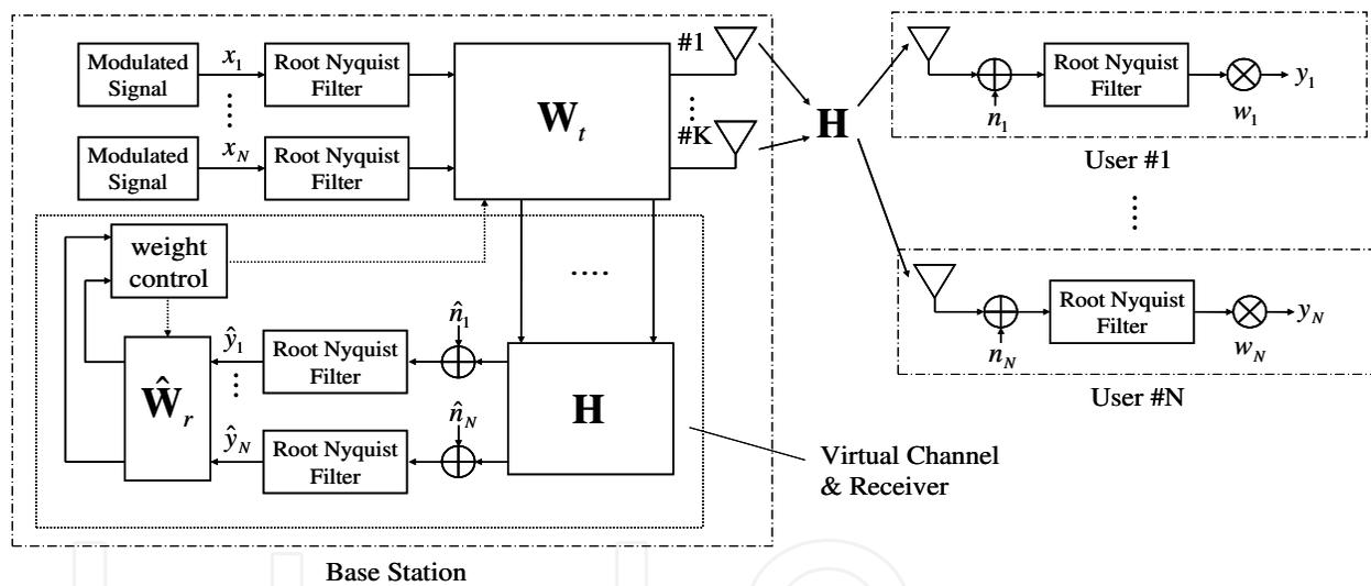
Fig. 12. System configurations
