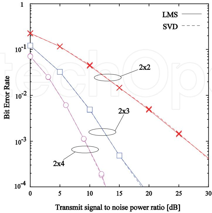
Fig. 8. Bit error rate performance (2 data stream,  $2 \times N_T$ )
