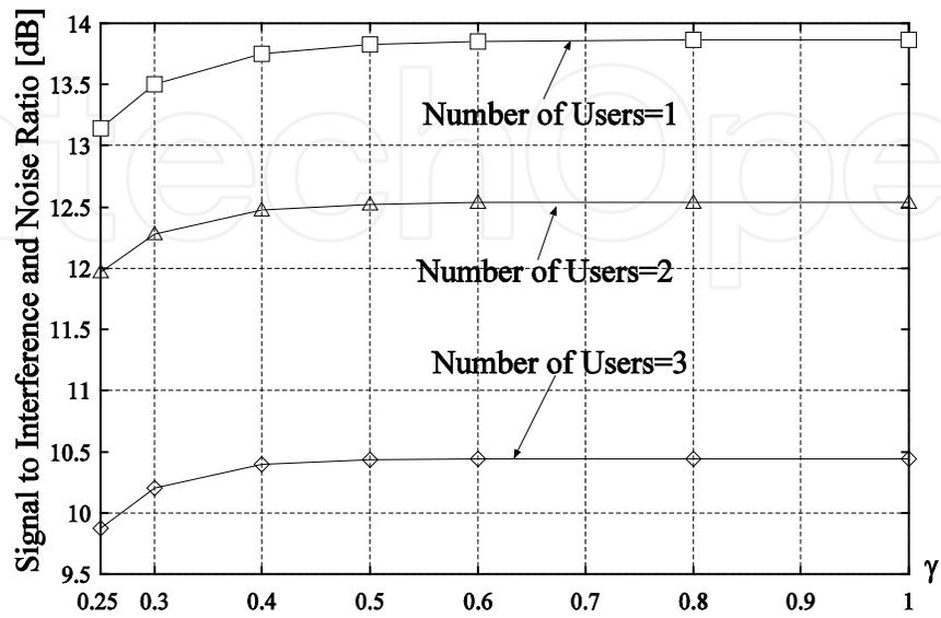
Fig. 15. SINR vs.  $\gamma$  ( $K=4$ ,  $SNR_{max}=10\text{dB}$ )
