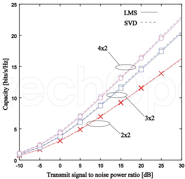
Fig. 9. Channel capacity performance ( $N_T \times 2$ )
