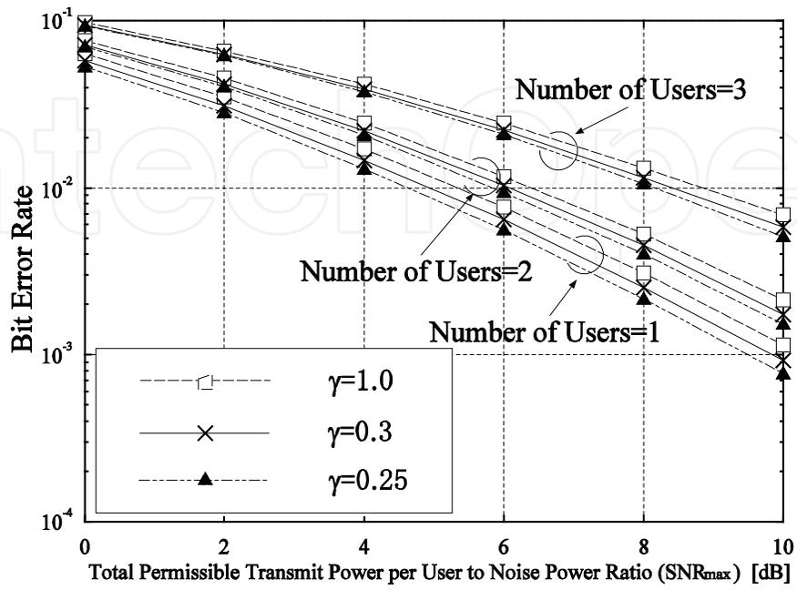
Fig. 17. Bit Error Rate Performance ( $K=4$ )
