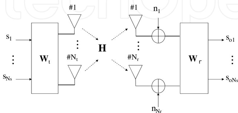
Fig. 1. MIMO System Model
