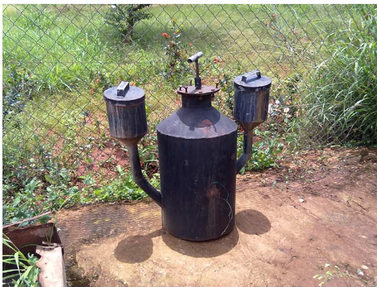
Fig. 1. 50L Capacity Metallic Prototype Biodigester
