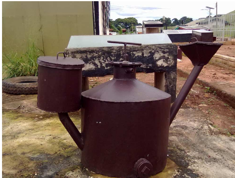
Fig. 2. 136L Capacity Metallic Prototype Biodigester
