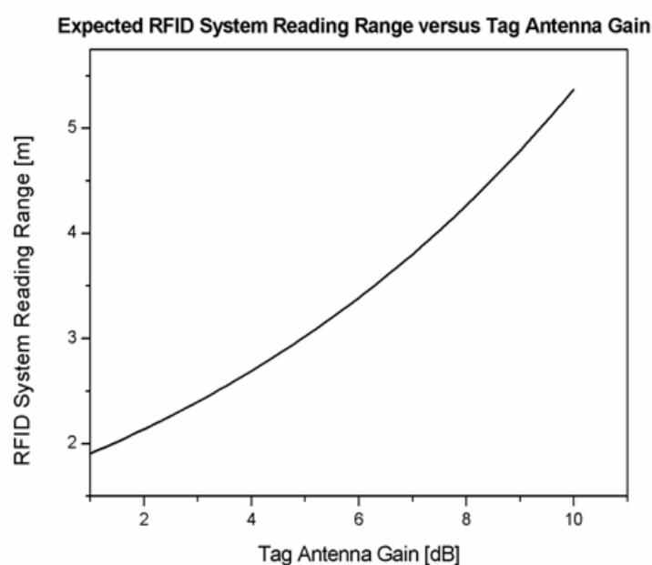
Fig. 3. Reading range versus tag antenna gain.
