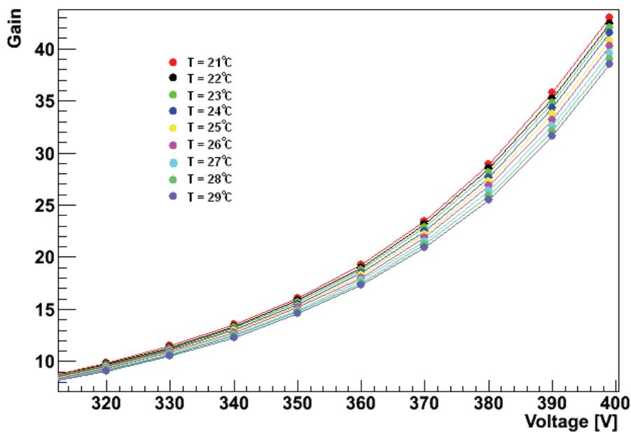
Fig. 4. Gain curves measured at different temperatures.
