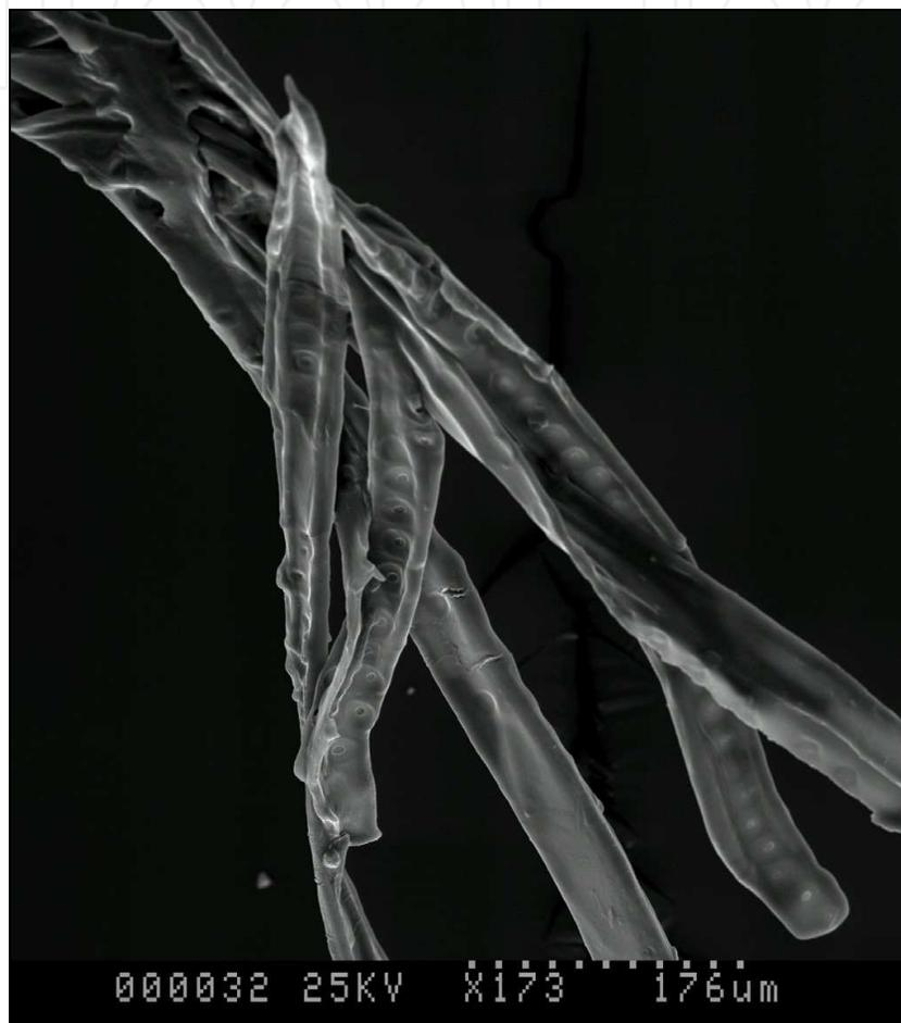
Fig. 7. Treated pine sapwood whose tracheids are easily manually disjoined. Softening and darkening are strongly related and both phenomena imply a lignin modification.
