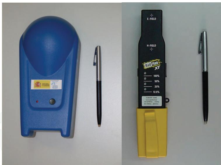
Fig. 1. Antennessa EME SPY and RadMan XT dosimeters
