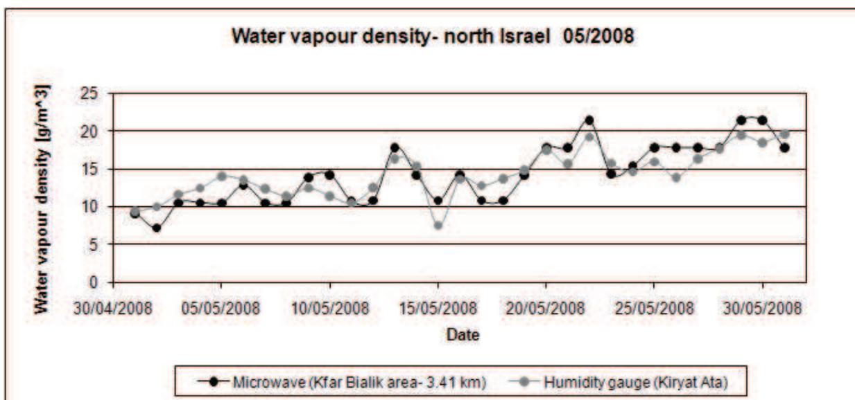
Fig. 2(b). Northern Israel - The humidity measurements were made, by the 3.41 km microwave link, during May 2008. The correlation between the two measurements is 0.87 with RMSD of 2 [g/m<sup>3</sup>]. Link's frequency: 22.05 GHz
