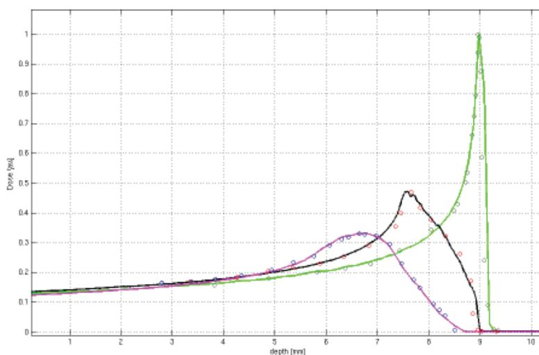
Fig. 7. Experimental measurements of carbon ion beam of 62MeV/u at Laboratori Nazionali del Sud (LNS) at the carbon ion beam line with and without ripple filters and compared to simulated curves.
