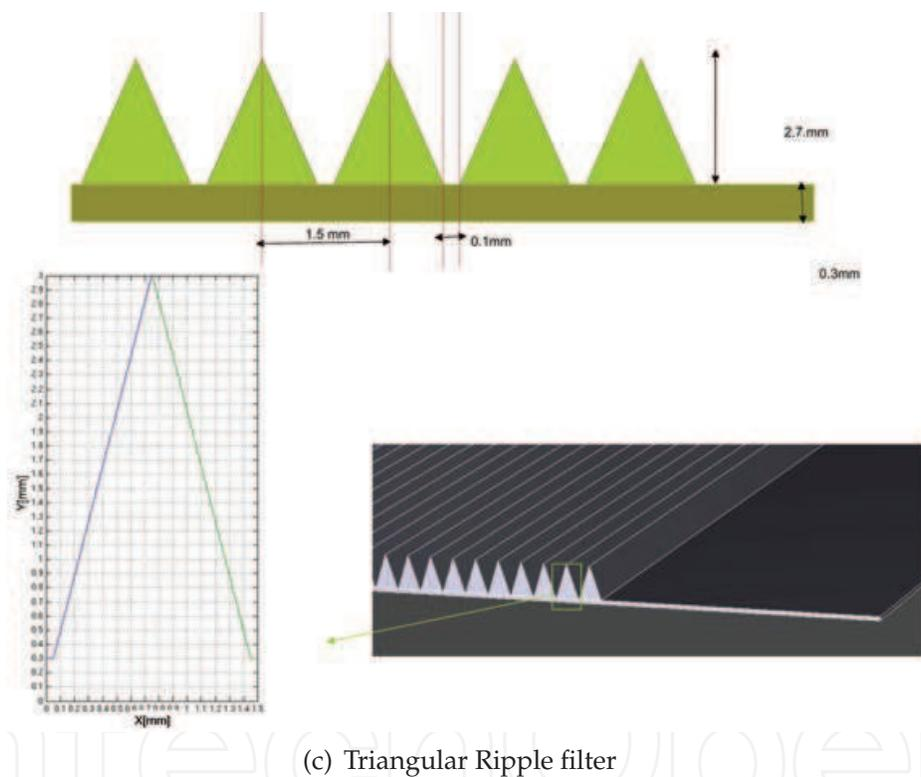
Fig. 3. Sections of ripple filters as described by (Weber and Kraft, 1999) of 3 mm (Type B) and the new triangular one (type A) and as designed and described in the Monte Carlo simulation with Geant4 (see also (Bourhaleb et al, 2008)).
