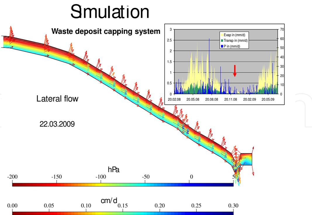
Fig. 9. Simulated hydraulic fluxes in a waste deposit capping system with the lateral flow situation
