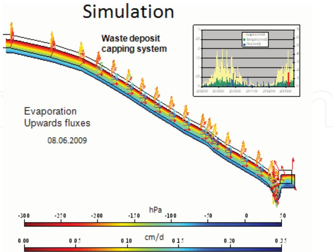
Fig. 8. Simulated hydraulic fluxes in a waste deposit capping system: the case presents situation with dominant upwards flow.
