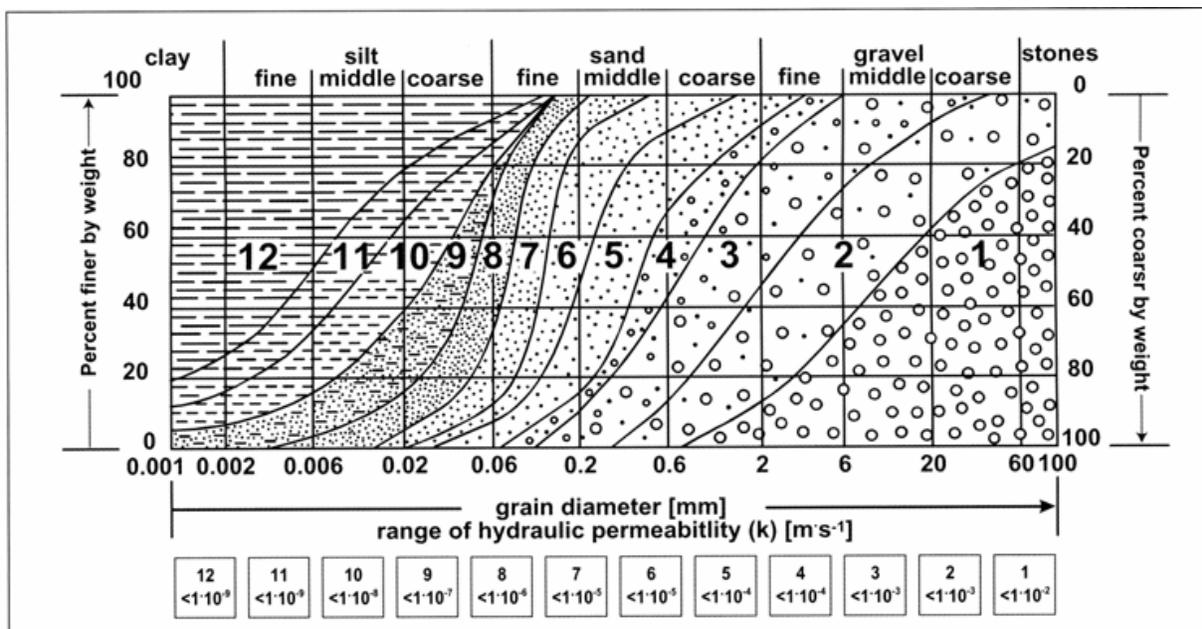
Fig. 1. Ranges of hydraulic permeability (expressed as  $k$  coefficient in  $\text{m}\cdot\text{s}^{-1}$ ) as related to grain-size distribution areas. The range of  $k \leq 10^{-7} \text{ m}\cdot\text{s}^{-1}$  is considered as an important barrier feature for mineral sealing in most of national regulations. Grain size distribution areas 10, 11 and 12 refer to this range. After Alamgir et al. (2005).
