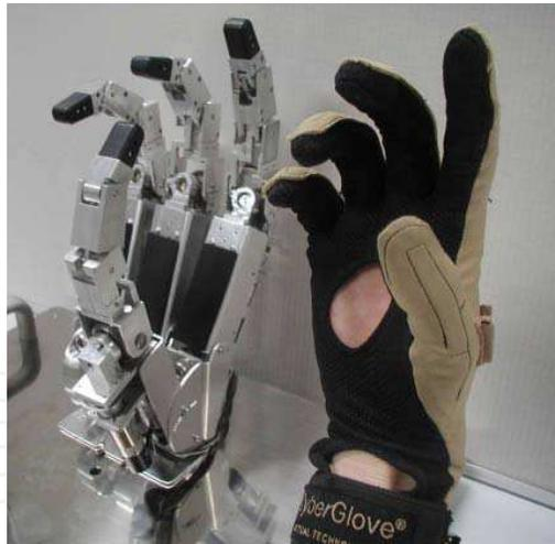
Fig. 10. A data glove controlling the joints motion of a robotic hand
