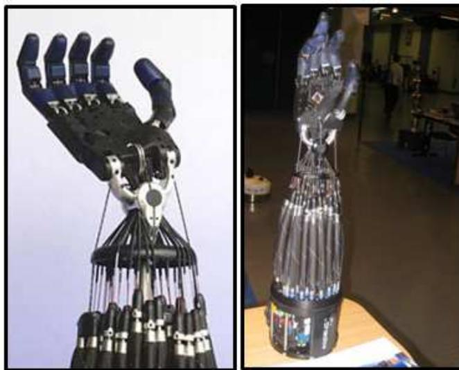
Fig. 6. The Shadow hand actuated with air muscles
