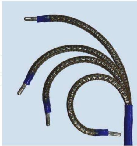
Fig. 4. A continuum manipulator with tendon actuation
