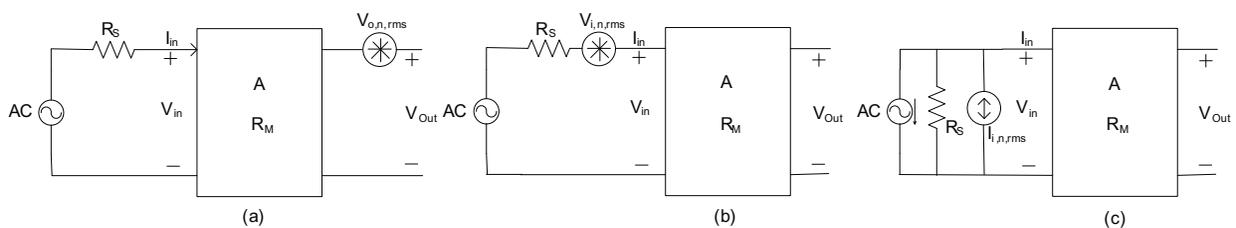
Fig. 6. (a) An amplifier with a gain factor of  $G$  ( $A$  or  $R_M$ ), and input impedance  $R_{in}$ , and the measured output noise  $V_{o,n,rms}$ ; (b) the input-referred noise as a voltage source; (c) the input-referred noise as a current source.
