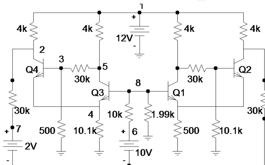
Fig. 27. A BJT circuit with multiple operational points
