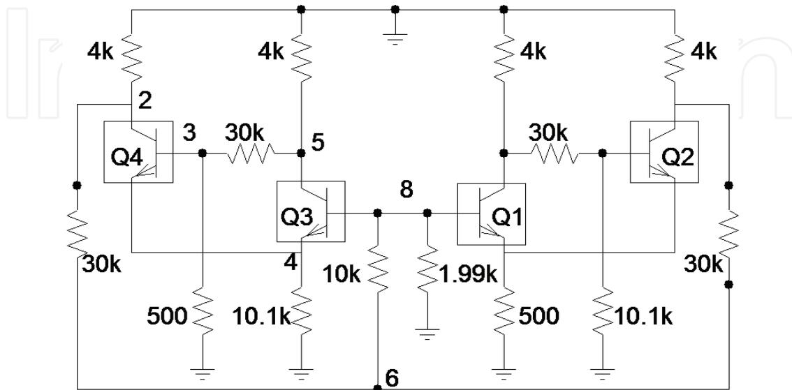
Fig. 28. The BJT circuit with locally biased transistors
