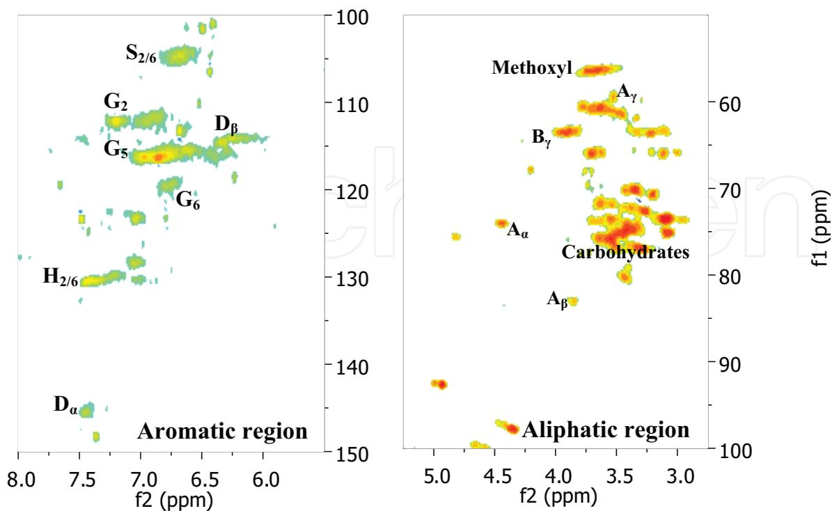
Fig. 6. (see correction 2) 2D HSQC spectra of switchgrass solution after dissolving 100 mg Wiley milled sample in 1:2 [Hpyr]Cl-d<sub>6</sub>/DMSO-d<sub>6</sub> (1.0 g) at 60 °C.
