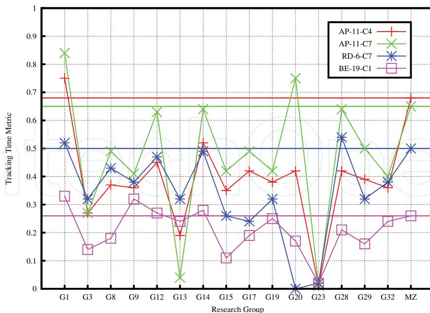
Fig. 9. Summary of results for the Tracking Time metric  $T_{Tracked}$  for the four analysed videos. The labels at the horizontal axis represent the identifiers for anonymous research groups participating to the evaluation, except for the **MZ** label, which represents the proposed tracking approach. Horizontal lines at the level of the obtained results for the proposed approach have been added to help in the comparison of results with other research groups.
