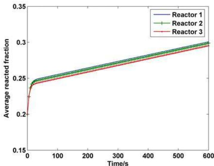
Fig. 11. The simulated hydrating rates for reactors 1, 2 and 3 while using air as heat transfer fluid
