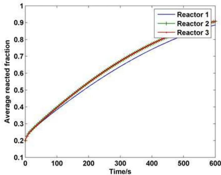
Fig. 10. The simulated hydrating rates for reactors 1, 2 and 3 with larger wall thickness
