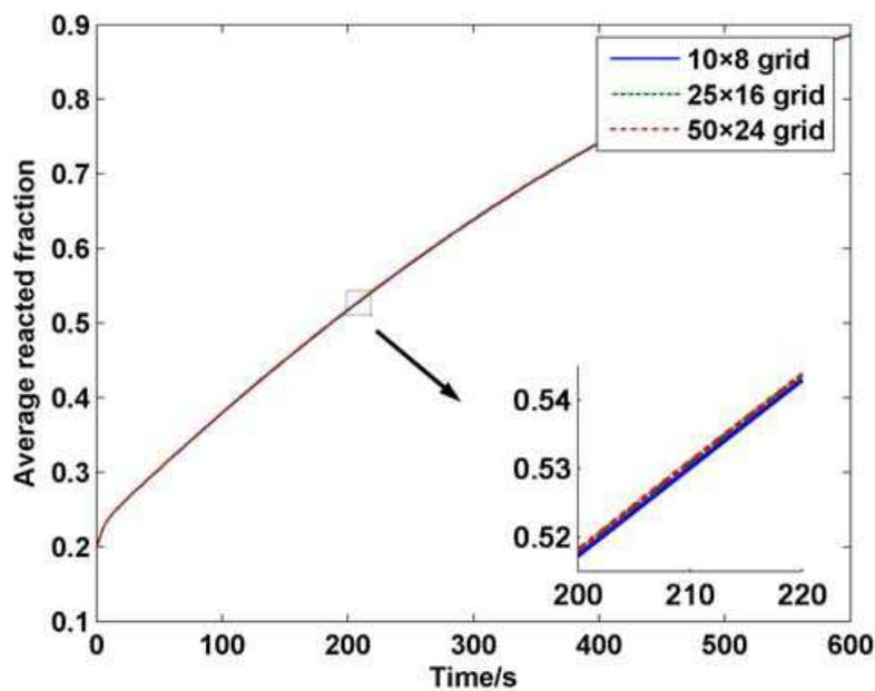
Fig. 4. The simulation results for grid independence test
