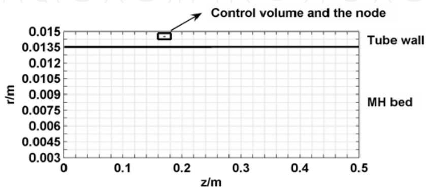
Fig. 2. The discretization of the computational domain
