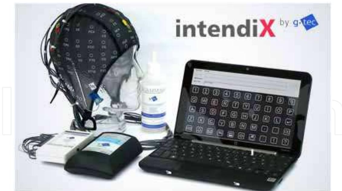
Fig. 12. IntendiX running on the laptop and active electrodes
