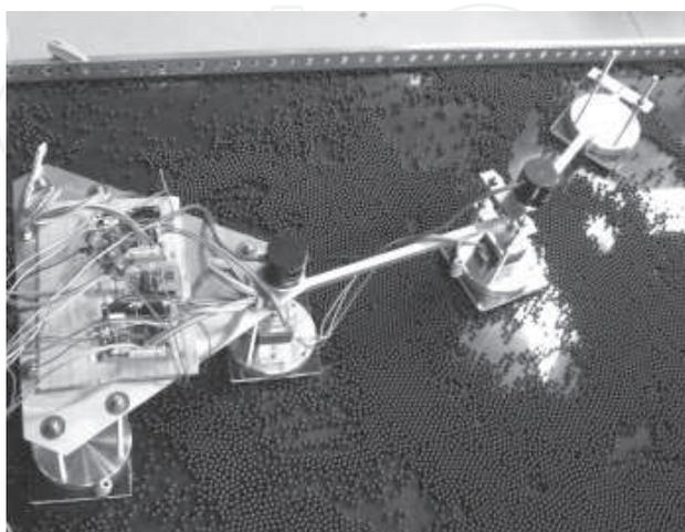
Fig. 13. Experimental apparatus for the planar two-link robot.
