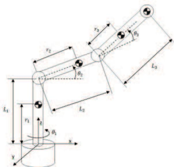
Fig. 1. Coordinate system of the 3D robotic manipulator
