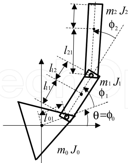
Fig. 7. Model of a Planar Two-Link Space Robot
