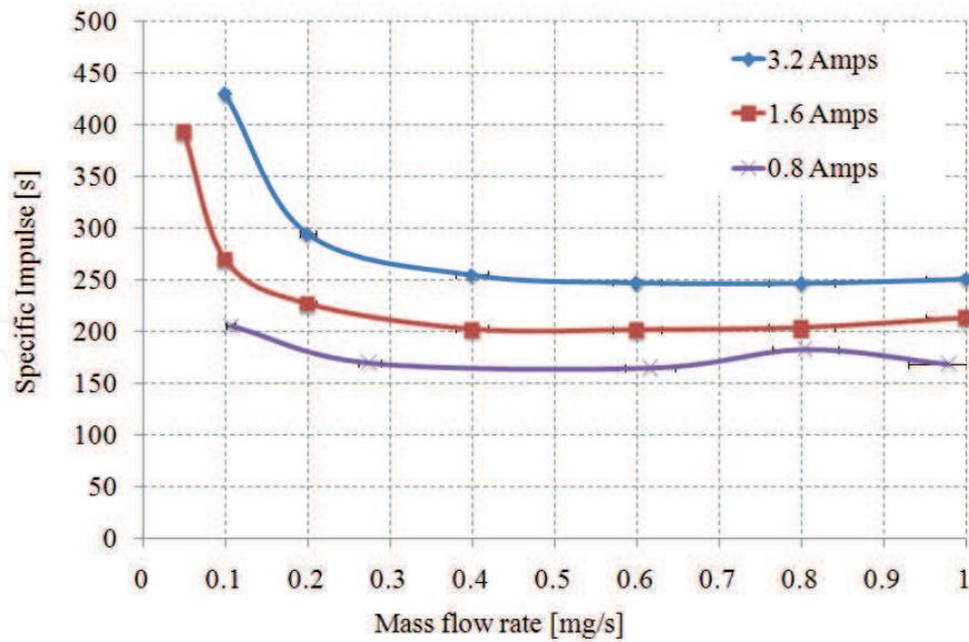
Fig. 7. Measurements of specific impulse with mass flowrate
