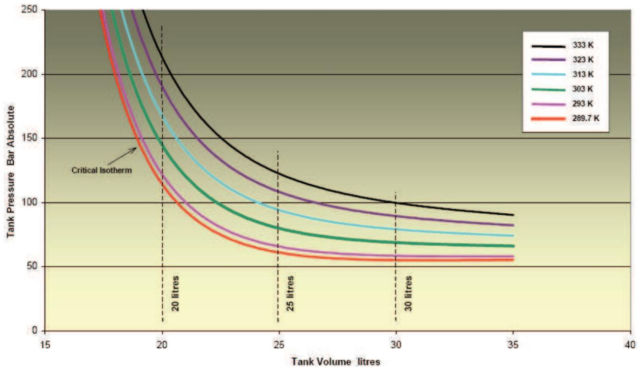
Fig. 12. Xenon isotherms for 30 Kg of Xenon
