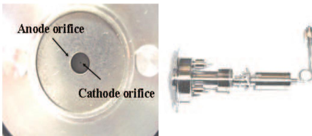
Fig. 6. T5 Hollow Cathode Thruster
