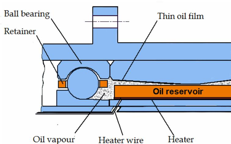
Fig. 11. Mechanism of oil transfer in static oil reservoir
