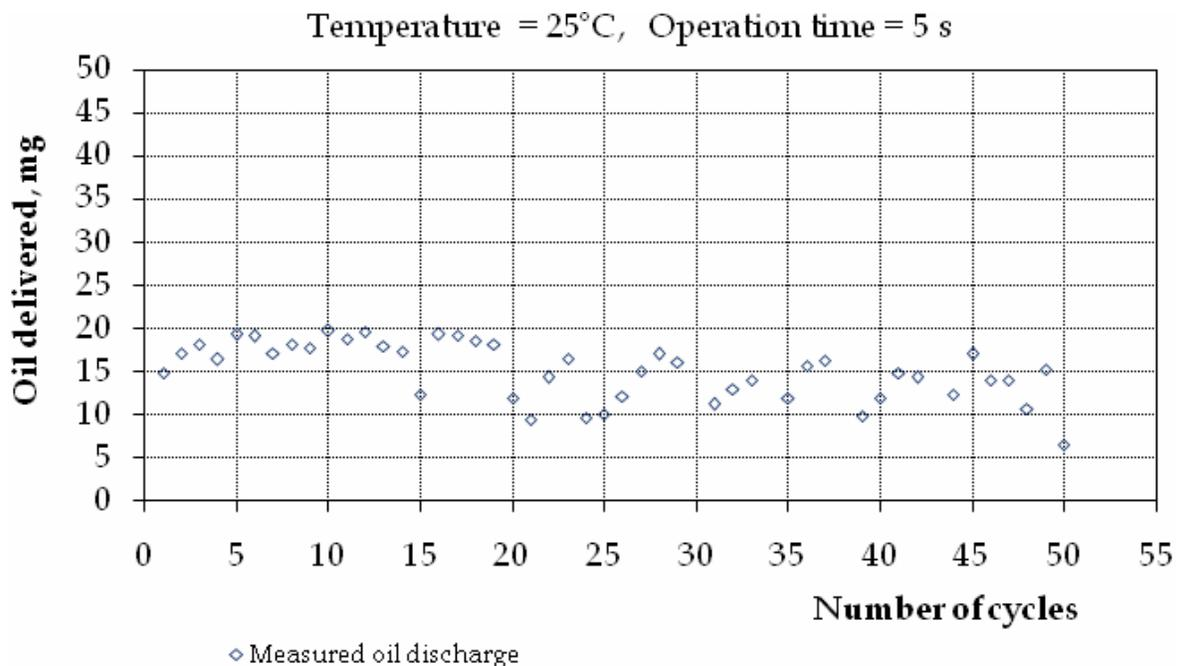
Fig. 10. Oil discharged by CLS for 50 cycles
