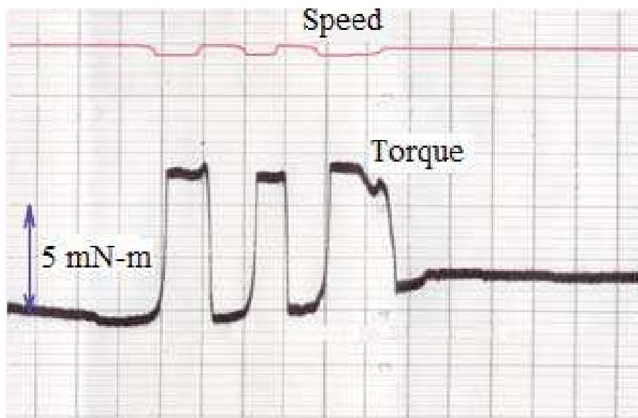
Fig. 5. Bearing friction torque variation due to retainer position change
