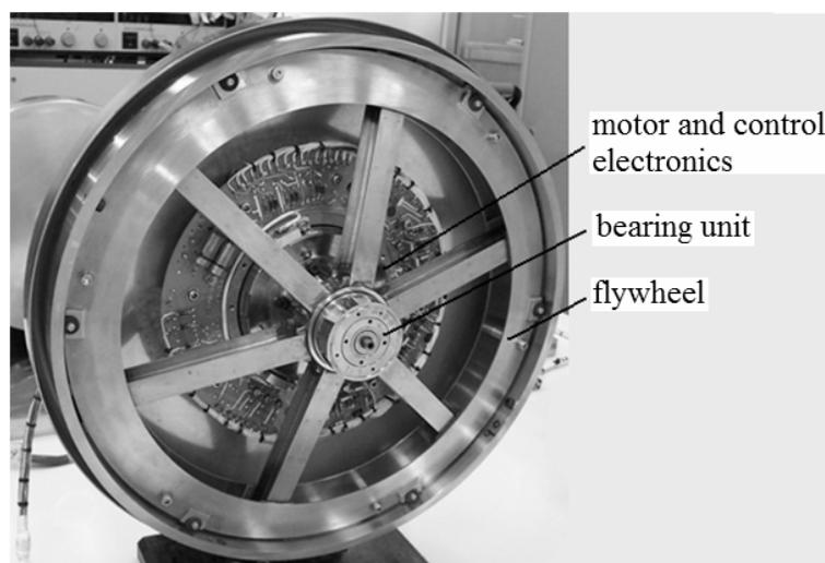
Fig. 1. Momentum wheel with top cover removed
