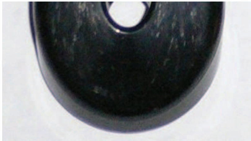
Fig. 3. Warpage and silver streaks at bottle Opener
