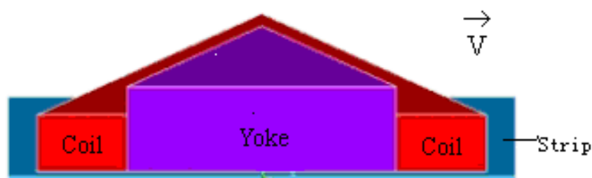
Fig. 1. New structure of the TFIH equipment
