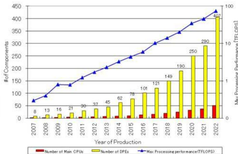
Fig. 2. Component density and maximum processing performance trends
