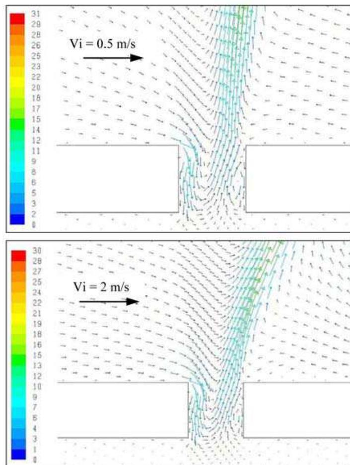
Fig. 9 Velocity vectors near the orifice at time  $t=T/2$  (maximum expulsion)
