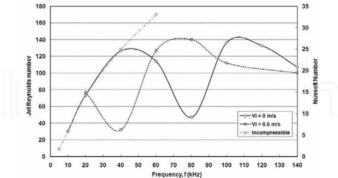
Fig. 18. Effect of compressibility on synthetic jet heat sink characteristics
