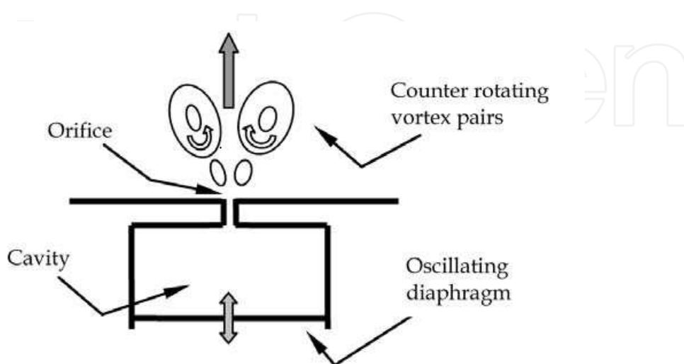
Fig. 3. Schematic diagram of a synthetic jet actuator
