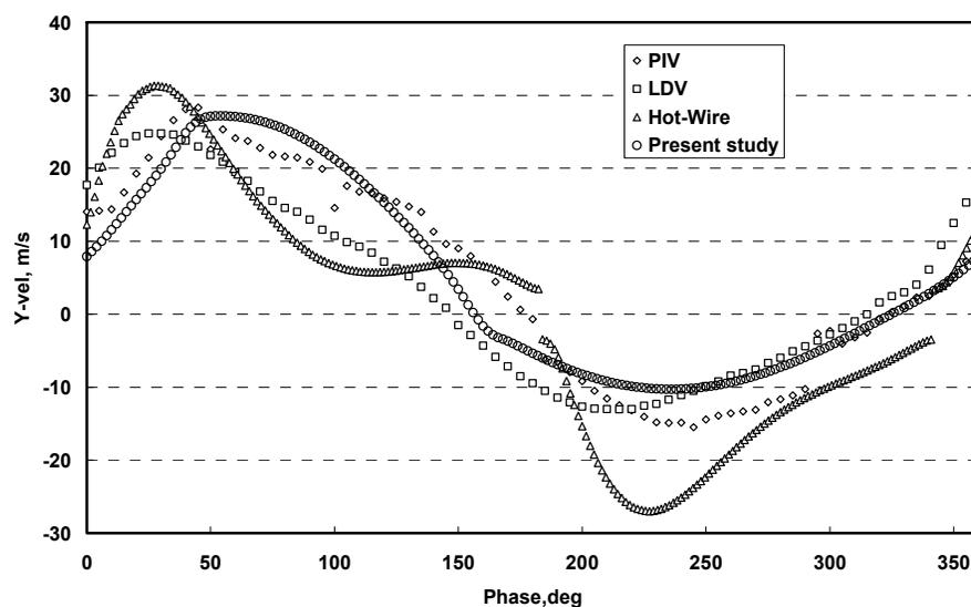
Fig. 6. Comparison of predicted axial/y-velocity of present work with the (PIV, LDV, Hot-wire) experimental data of (Yao et.al., 2006) at 0.1 mm from the orifice exit plane ( $f = 444.7$  Hz,  $A=1.25$  mm)
