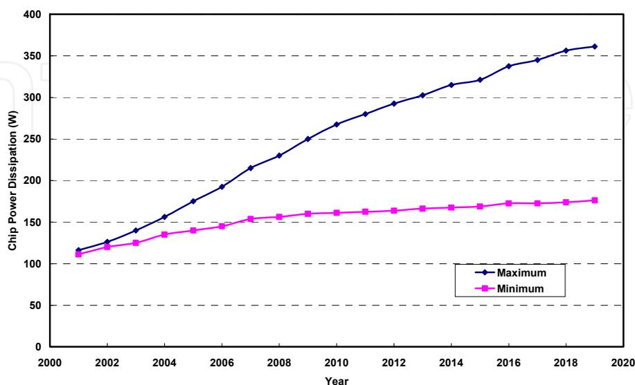
Fig. 1. Evolution of chip power dissipation (Chu, 2003)
