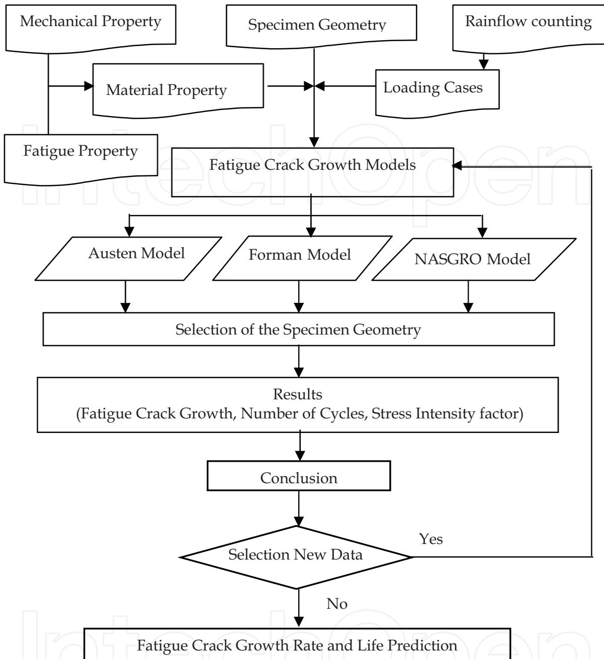
Fig. 5. Flow chart of the simulation process
