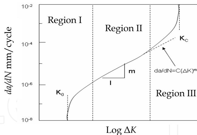
Fig. 2. Typical  $da/dN$  versus  $dK$  curve
