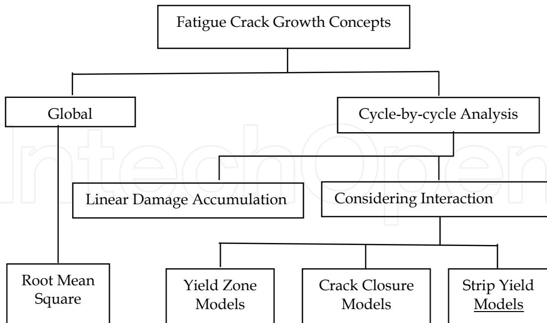
Fig. 1. Classification of the fatigue crack growth concepts
