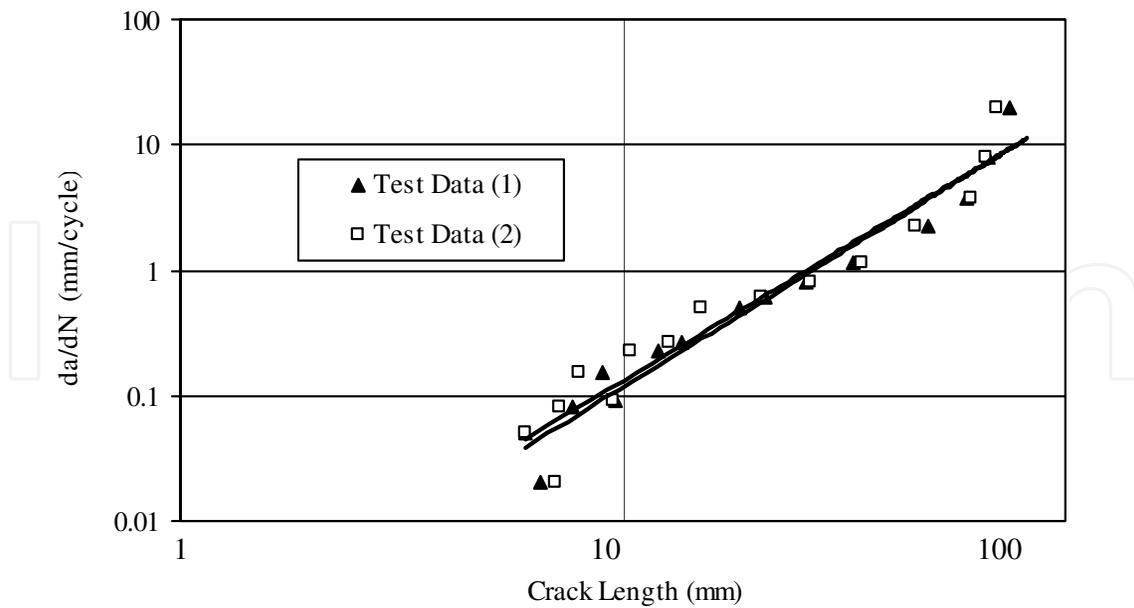
Fig. 9. Fatigue crack growth rate versus crack length of test data under load cases 1 and 2
