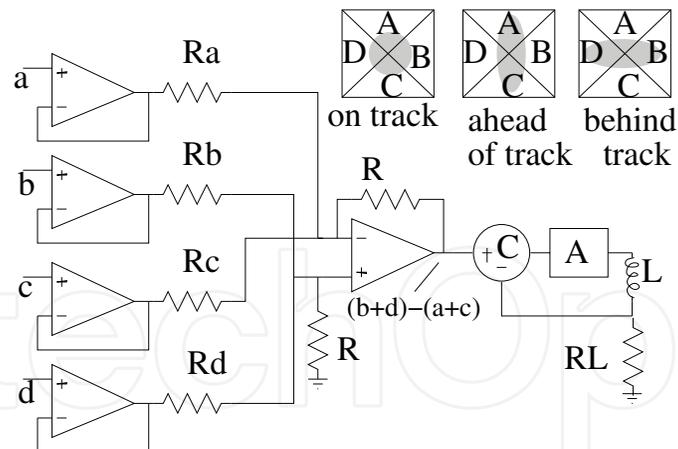
Fig. 11. Focus electrical subsystem.
