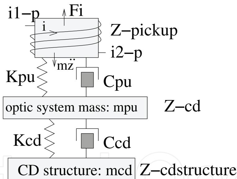
Fig. 10. Mechanical model of the CD structure.
