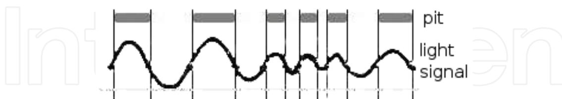
Fig. 12. Example of the EFM modulated light signal received by the photo-diodes when the track reflects back the laser light.
