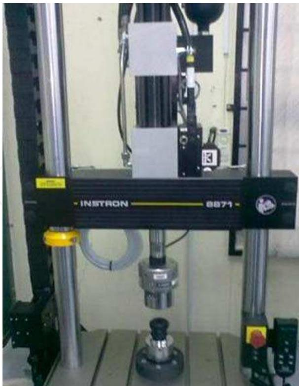
Fig. 4. Instron 8871 table top model fatigue systems
