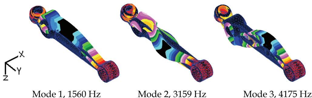
Fig. 12. Simulated modal frequencies and mode shapes from FEA
