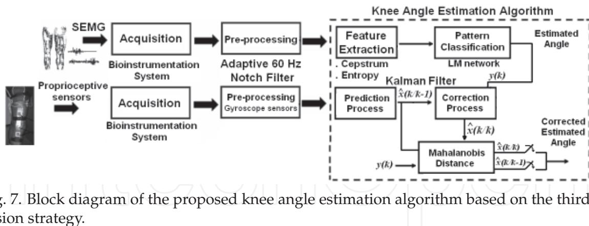
Fig. 7. Block diagram of the proposed knee angle estimation algorithm based on the third fusion strategy.
