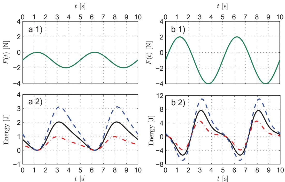
Fig. 5. The internal energies within two periods of the driving. The solid black line shows the energy  $E(t)$ , the dashed blue line depicts  $E_R(t)$  and the dot-dashed red line illustrates  $E_L(t)$ . In the panels a1) and a2) we take  $F_1 = 1.0$  N, in the panels b1) and b2) we take  $F_1 = 3.0$  N. The static component ( $F_0 = -1.0$  N), the frequency ( $\omega = 0.4\pi\text{s}^{-1}$ ), and the diffusion constant ( $D = 1.0\text{m}^2\text{s}^{-1}$ ) are the same in all panels.
