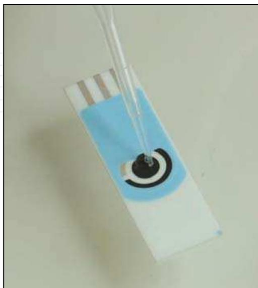
Fig. 8. Screen printed electrode used for biomediator immobilization.
